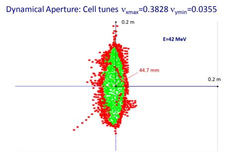
Some of the losses (red) are at smaller amplitudes enclosed inside the overall accepted region. So, the Muon1 study counted the entire green area and did not see the losses at low amplitudes that actually dictate the safe amplitudes for beams. It is planned to rerun the Muon1 study with an updated dynamic aperture definition at a later date.
