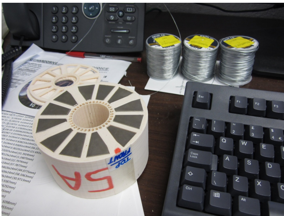
Figure 31: The pieces of the eRHIC LDRD Halbach magnet placed in a new 3D-printed holder to form magnet “5A”. This is a corrected Halbach quadrupole whose holder incorporates holes for iron shims to be placed around the inside of the bore (iron wire grades shown in background).
