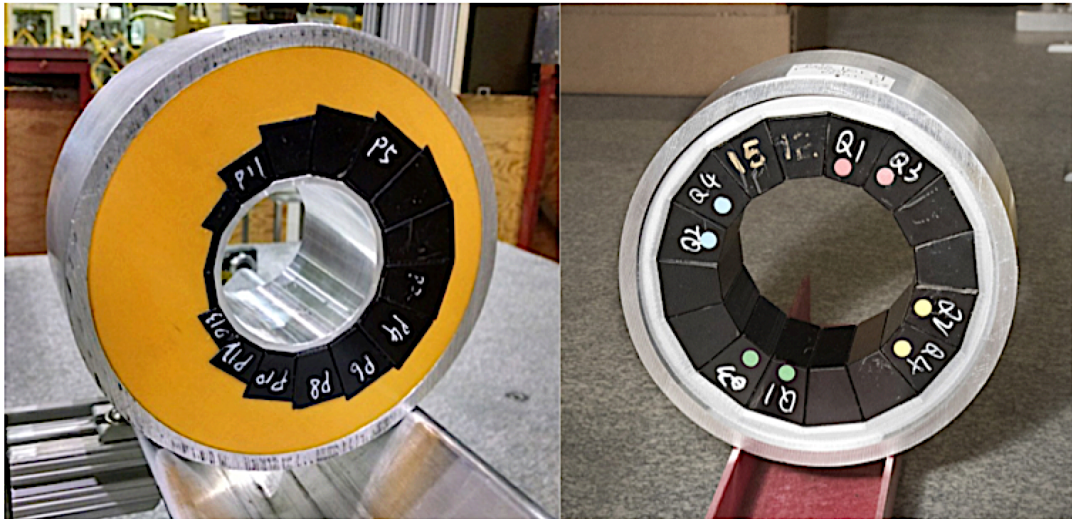
Figure 10: Defocusing (left) and focusing (right) Halbach prototype magnets for CBETA E_{\max}=250 MeV.
