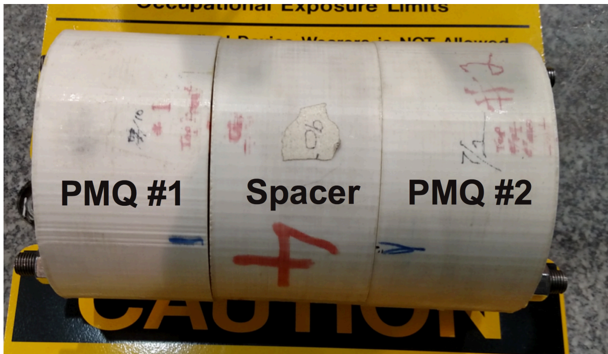
Figure 35: Layout of the set-up for measuring the cross talk between the two Halbach magnets PMQ#1 and PMQ#2, where the 6 mm long spacer made of plastic is placed between.
