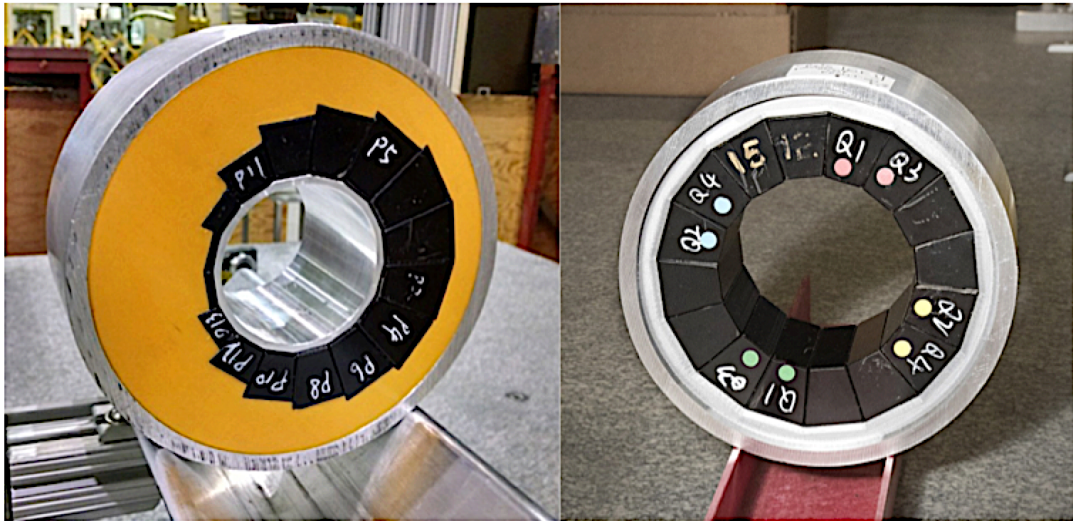
Figure 10: Defocusing (left) and focusing (right) Halbach prototype magnets for CBETA E_{\max}=250 MeV.
