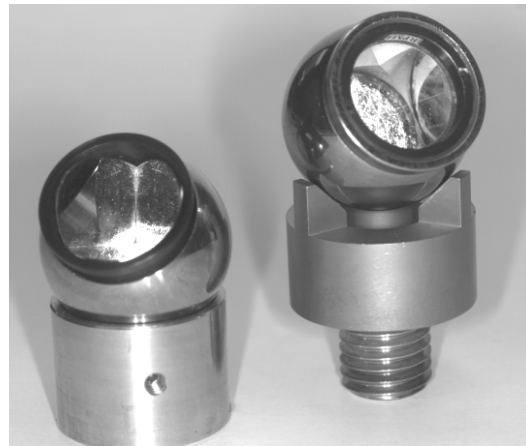
Figure 2: Sphere mounted glass and air
