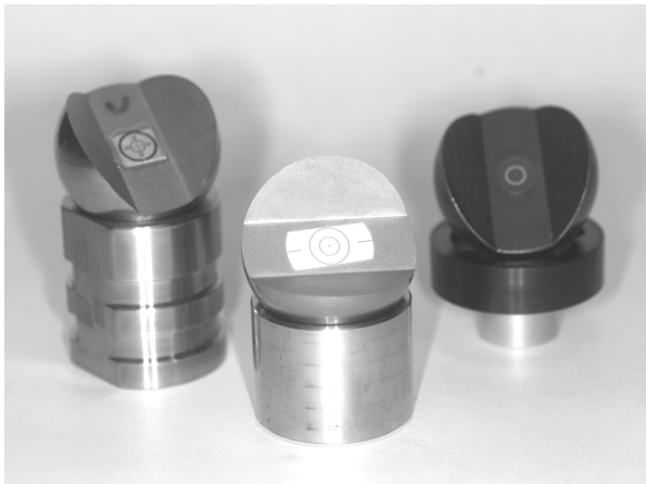
Figure 1: Sphere mounted theodolite target
