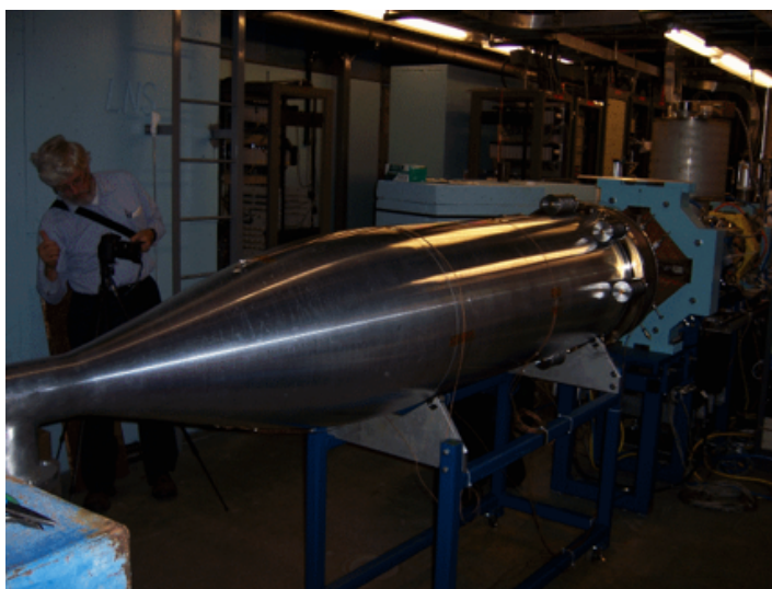
Figure 4.6.2: The completed beam dump before installation of the shielding blocks.
