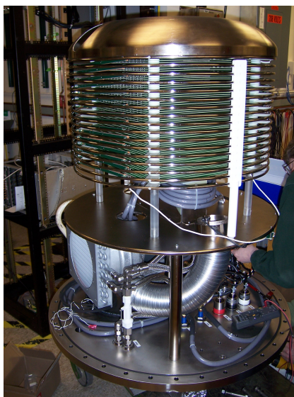
Figure 4.2.4: The HV section of the 750kV power supply. Individual circuit boards are visible inside the potential grading rings. The primary winding of the insulating core transformer is the large diameter gray-insulated wire below the circuit boards. The HV section is mounted in the pressurized \text{SF}_6 tank with its axis parallel to the axis of the gun ceramic.
