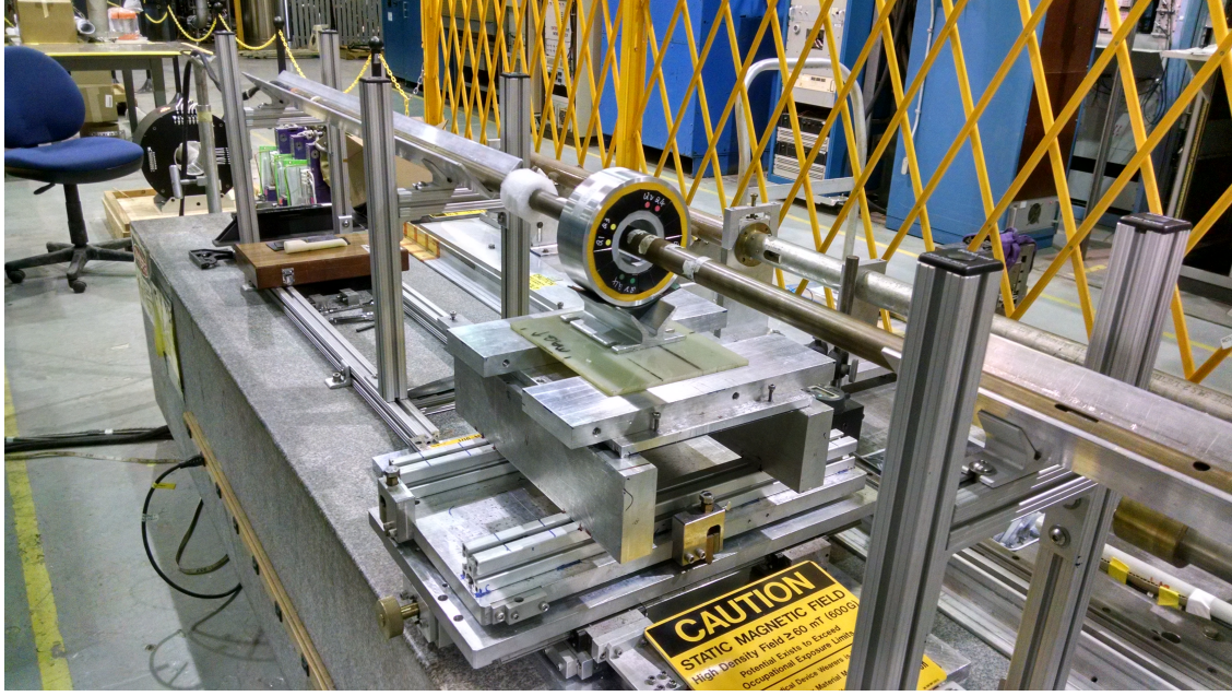
Figure 3.1.9: A prototype QF Halbach magnet being measured on BNL's rotating coil.
