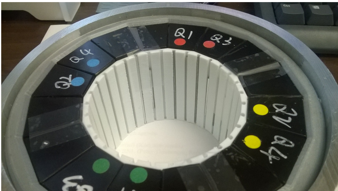
Figure 3.1.8: A shimmed prototype QF Halbach magnet, showing the 3D printed plastic shim holder (white) containing iron wires.
