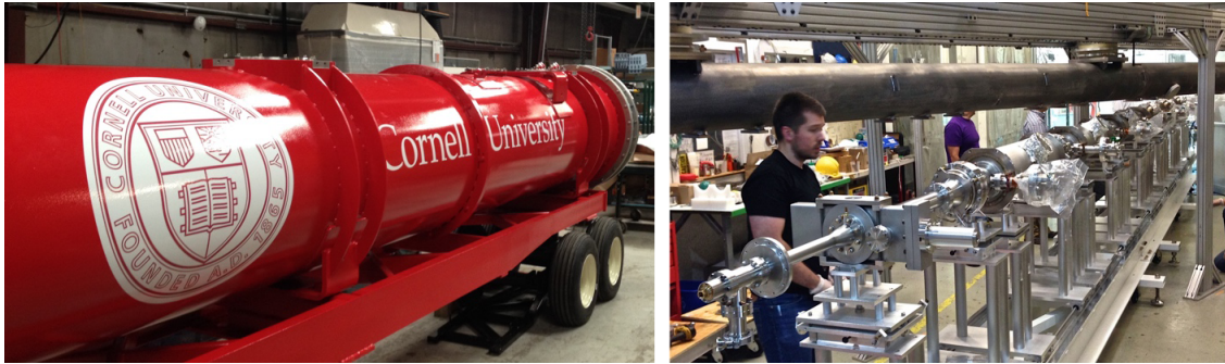
Figure 5.4.4: Left: Vacuum Vessel as received by Cornell University. Right: Marriage step: the cavity string coming from the clean room assembly is rolled under the HGRP providing precision alignment.
