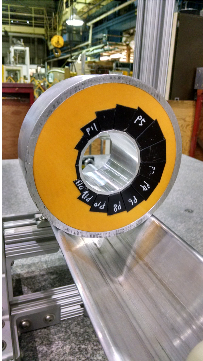
Figure 3.1.6: An unshimmed prototype BD magnet awaiting measurement at BNL.
