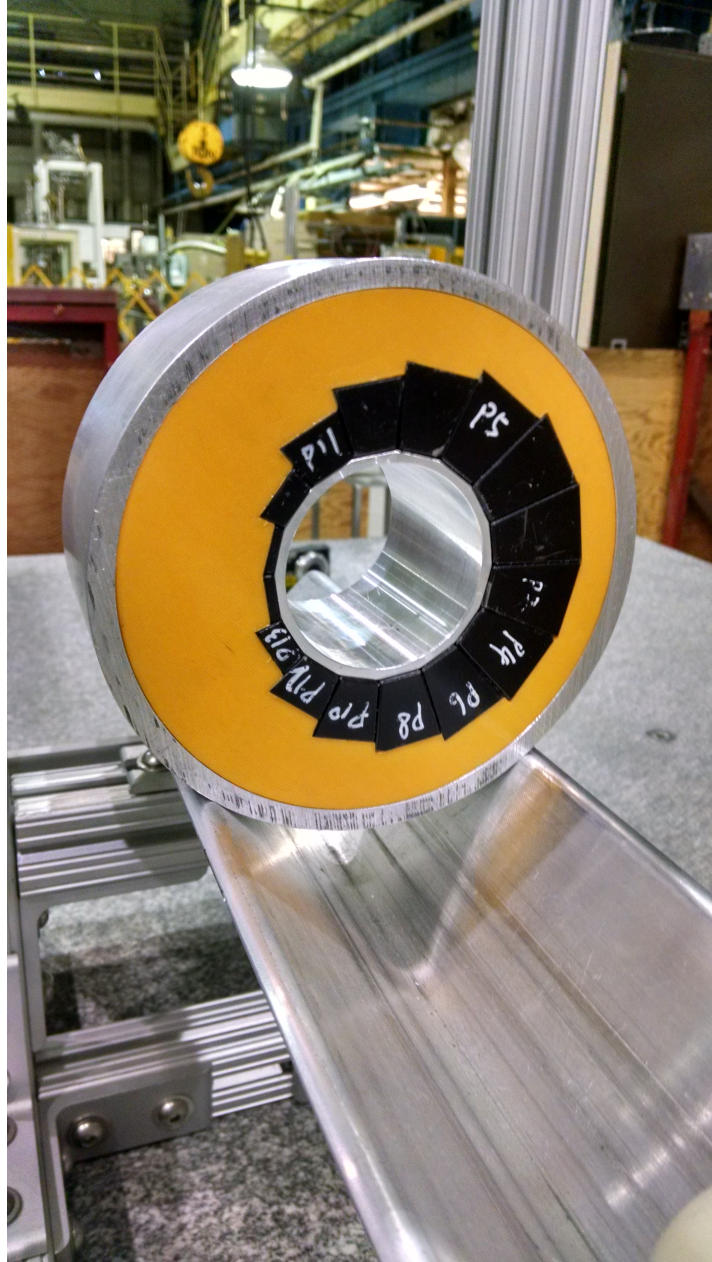
Figure 3.1.6: An unshimmed prototype BD magnet awaiting measurement at BNL.
