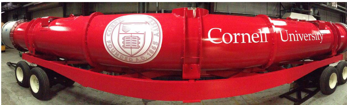
Figure 6 The full-scale prototype 1300 MHz cryomodule that is available for C \beta use.
