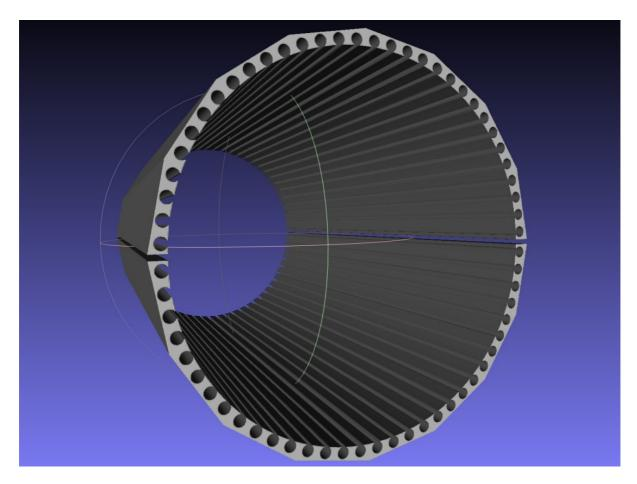
There are two types of Halbach magnet bore in CBETA: 108 QF-type magnets and 108 BD-type magnets. Their dimensions are shown in the table below, consistent with v6/v6.5 of the CBETA Halbach magnet designs.
