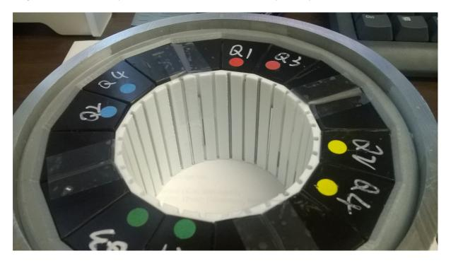
Note that the holder can be made of any non-magnetic material and that the holder pictured above has only 32 slots for wires, fewer than in the final version. The picture below shows a CBETA "first girder" magnet undergoing rotating coil measurement while containing a plastic wire holder.
