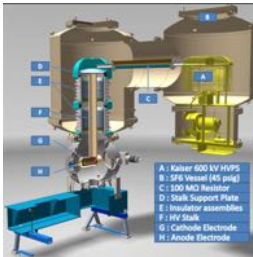
Figure 4.2.1: A cutaway view of the DC photoemission gun. Photocathodes are prepared in a load lock system mounted on the large flange at the left, and transported through the cathode cylinder to the operating position in the Pierce electrode shape on the right. The beam exits through the small flange to the right.
