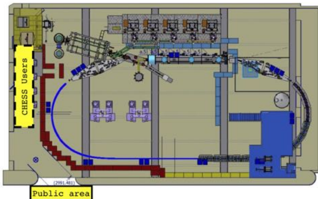
Figure 9.3.1: A candidate layout for the baseline shielding configuration.
