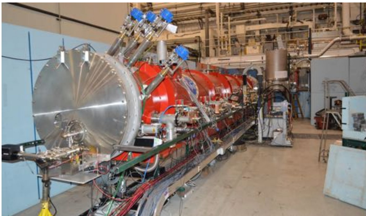
Figure 1.3.3: The Cornell Main Linac Cryomodule (MLC) installed for RF testing in the experimental hall L0E.
