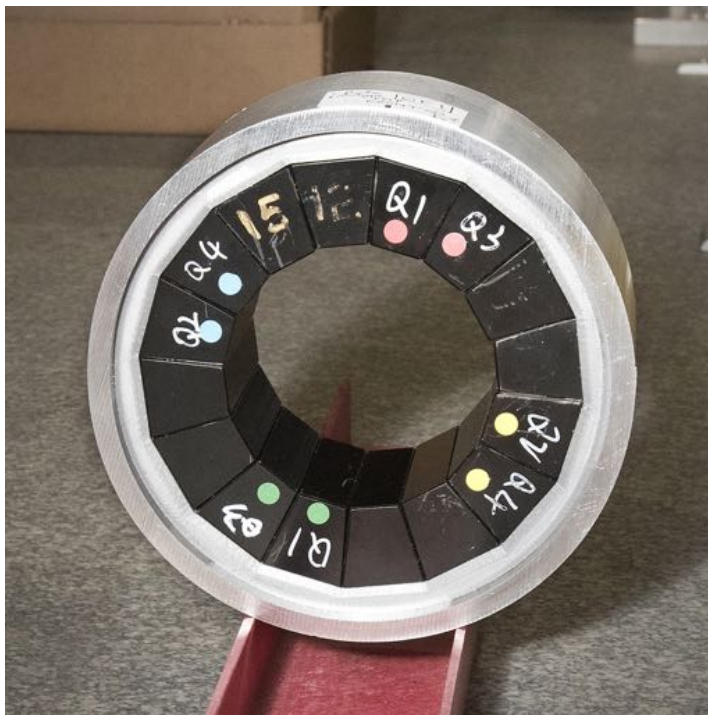
Figure 3.1.7: An unshimmed prototype QF (pure quadrupole) Halbach magnet.
