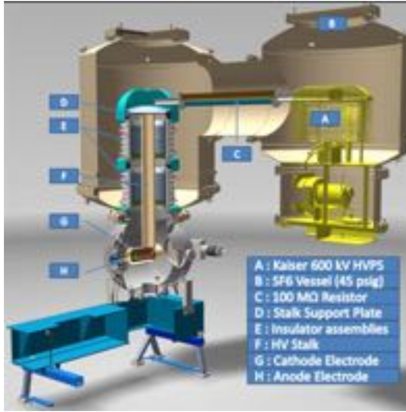
Figure 1.3.1: A cutaway view of the DC photoemission gun. Photocathodes are prepared in a load lock system mounted on the large flange at the left, and transported through the cathode cylinder to the operating position in the Pierce electrode shape on the right. The beam exits through the small flange to the right.
