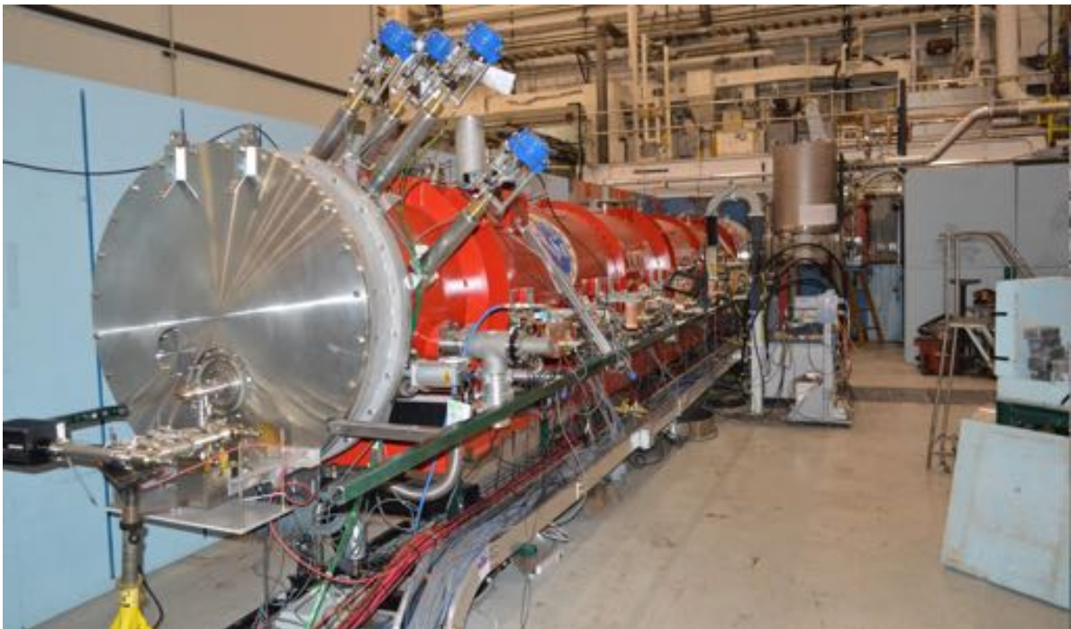
Figure 5.1.1: The Cornell Main Linac Cryomodule (MLC) installed for RF testing at Cornell.
