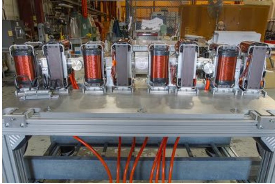
Figure 1.5.1: The prototype FFAG girder with 8 Halbach magnets, its vacuum chamber, cooling and beam diagnostics ports.
