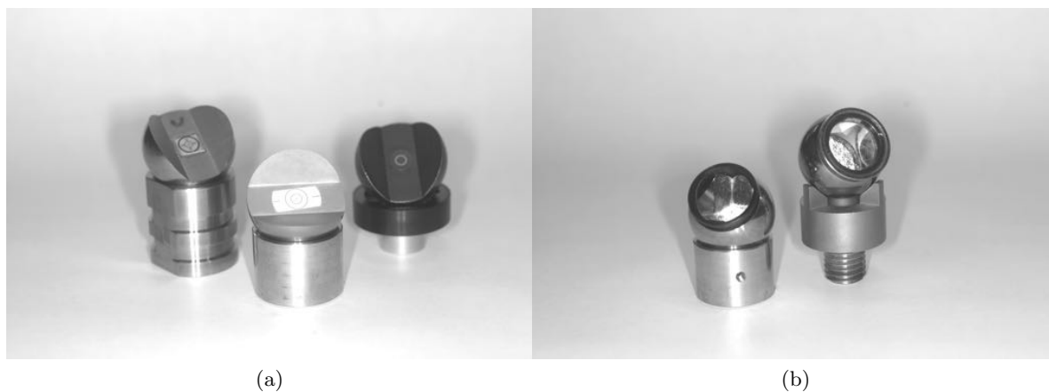
Figure 11.1.1: Left: Sphere mounted theodolite target. Right: Sphere mounted glass and air reflectors.
