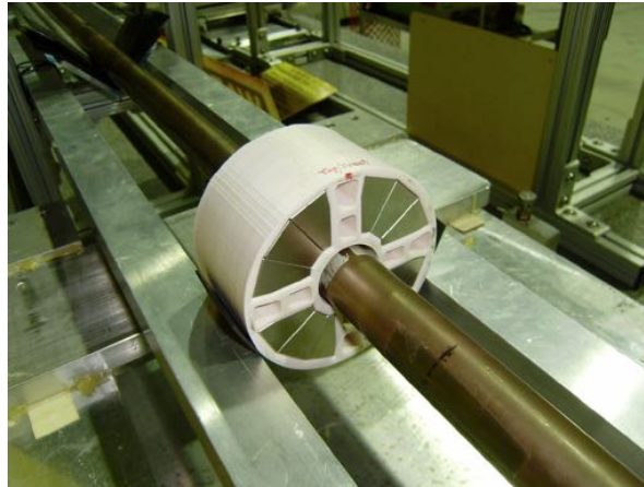
Figure 2.7.2: A prototype eRHIC Halbach style quadrupole, with an open mid-plane that allows synchrotron radiation to escape.
