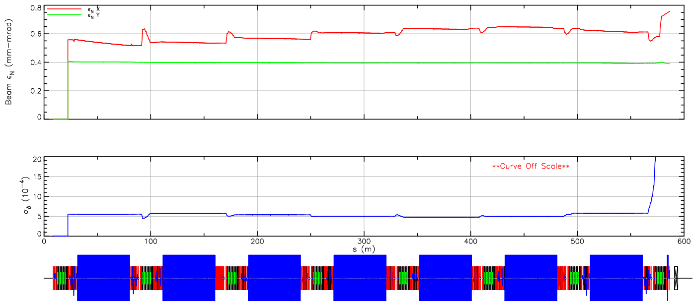
Figure 4: Normalized beam emittance and energy spread through 4-pass energy recovery.
