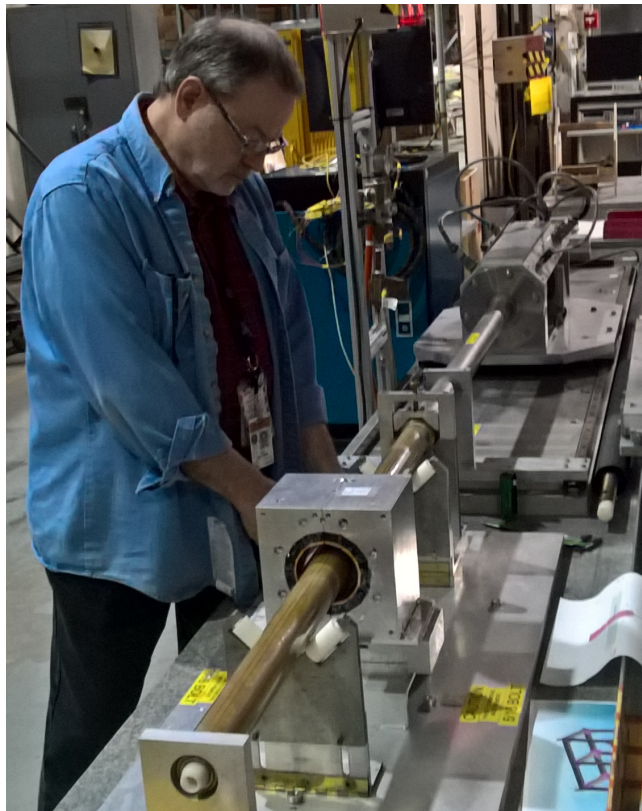
Figure 8: John Cintorino operates a rotating coil at BNL to measure the multipoles of a QF magnet (bottom center).
