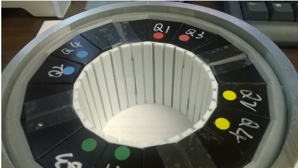
Figure 39: The above magnet is part of a prototype series of 6 quadrupole and 6 combined-function magnets, which have been shimmed to field quality required for CBETA, as described in other documents.
