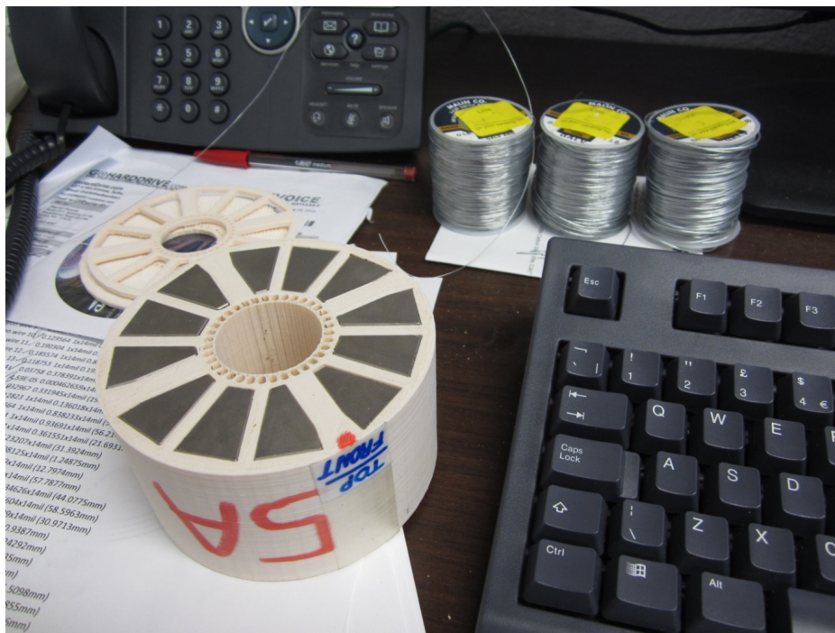
Figure 31: The pieces of the eRHIC LDRD Halbach magnet placed in a new 3D-printed holder to form magnet “5A”. This is a corrected Halbach quadrupole whose holder incorporates holes for iron shims to be placed around the inside of the bore (iron wire grades shown in background).
