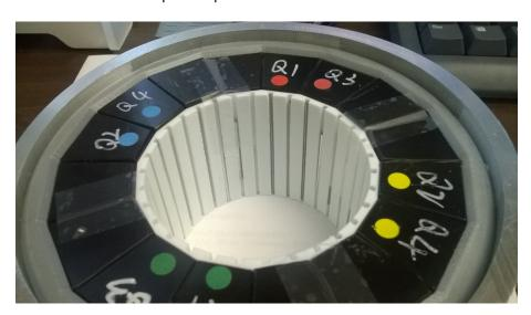
The above magnet is part of a prototype series of 6 quadrupole and 6 combined-function magnets, which have been shimmed to field quality required for CBETA, as described in other documents.
