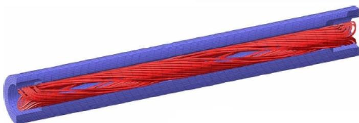
Figure 2: The 360°-twist helix module model in OPERA.
