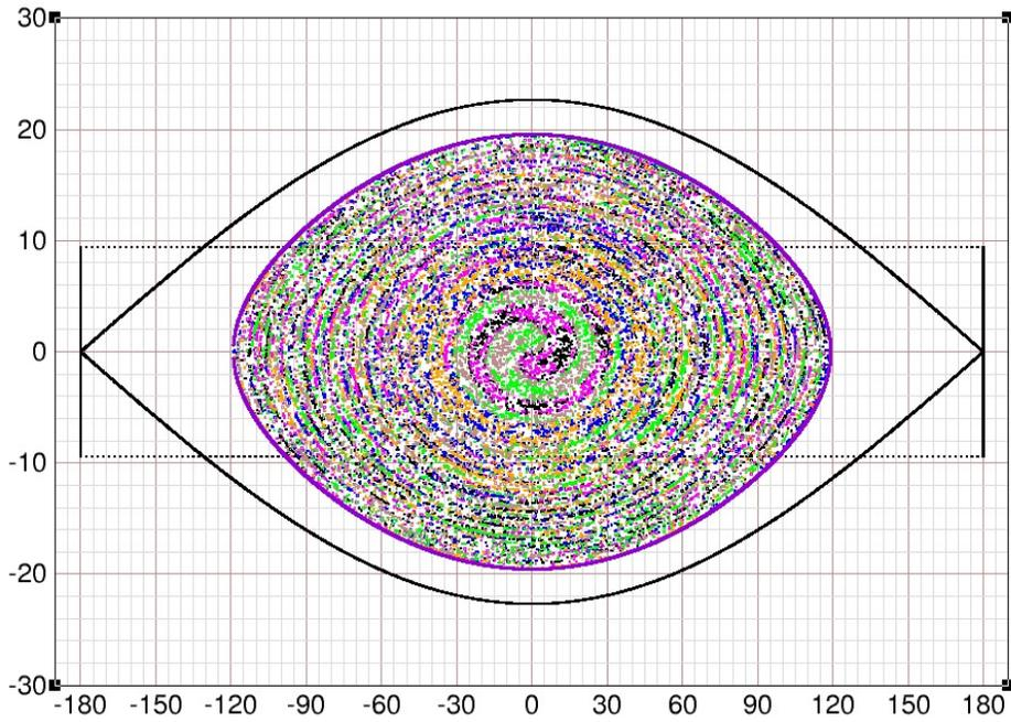
Figure 14: Completion of 3 to 1 merge. Time = 120 ms. The violet border enclosing the bunch is matched to the bucket. The area inside the border is  $0.612 \text{ eV*s/A}$ . This gives a growth factor of  $0.612/0.60 = 1.02$ .
