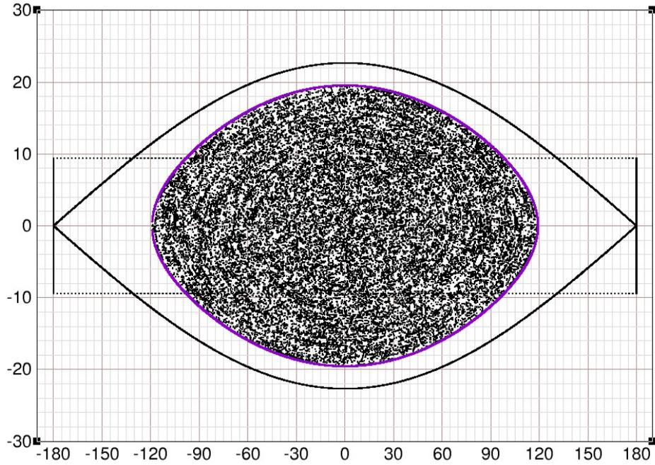
Figure 16: Merged bunch of Figure 14 with color suppressed. This is the **start of harmonic 8 squeeze**. As already mentioned, the total emittance of the 6 bunches that were merged to make this bunch is  $0.60 \text{ eV*s/A}$ . The violet border enclosing the bunch is matched to the bucket. The area inside the border is  $0.612 \text{ eV*s/A}$ , which gives a growth factor of  $0.612/0.60 = 1.02$ . Note also that the fractional momentum spread of the bunch is  $\Delta p/p = \pm 0.0016$ .
