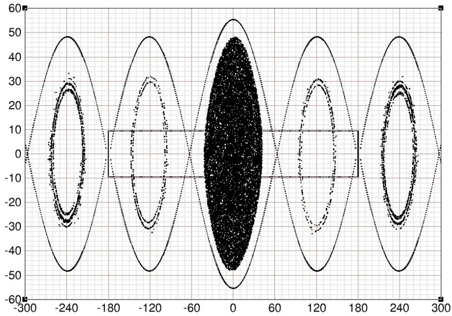
Figure 25: **End of harmonic 12 squeeze** showing all satellite bunches. A total of 12.95 percent of the particles in the initial merged bunch end up in satellite buckets with 3.42 percent in the two inner satellite and 9.53 percent in the two outer satellite buckets. The fractional momentum spread of the central bunch is  $\Delta p/p = \pm 0.0039$ .
