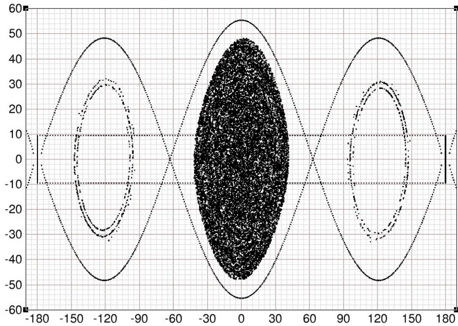
Figure 24: **End of harmonic 12 squeeze.** As already mentioned, the squeeze is done by raising the harmonic 12 voltage linearly from 0 to 180 kV over a period of 10 ms. The harmonic 4 and 8 voltages are held constant at 12 and 22 kV, respectively, during this time. Two of the four satellite bunches formed during the squeeze are shown.
