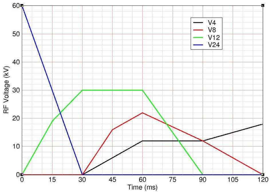
Figure 33: Consider now the voltage program shown above. Here, during the interval from 90 to 120 ms, the harmonic 4 voltage is raised from 12 to 18 kV. The voltage is held at this value during the squeeze of the merged bunch. The resulting plots of satellite bunch percentage and squeezed bunch emittance are given in the next two figures.
