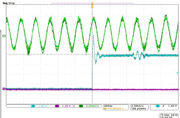
To correct the rf pickup we added active background subtraction in the manager. Each measurement now uses two machine cycles. One is done normally and one is done with the electron gate turned off. The "off" data are subtracted from the "on" data to produce a complete profile data set. An example of this is shown in the two figures below. The left figure shows the baseline with no beam and rf subtraction and the right figure shows a beam profile with background subtraction.
