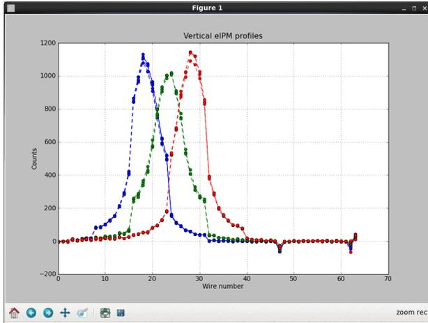
The figure above shows profiles of the beam with the beam in three positions in the vertical eIPM. There is a gain step between 8-channel amplifier boards and the size of the step increases as the profile amplitude gets larger. This behavior results in a position-dependent emittance as shown below. Here we plot the measured  $\sigma^2$  vs. position of the center of the beam. This 8-channel gaps in the profile measurements was not seen in the rest Run 16 and it is not understood.
