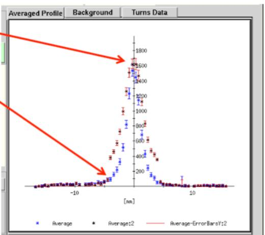
This pattern of profiles discontinuities at the breaks between the 8-channel amplifier groupings with the rf on appeared across the entire eIPM as shown here. The left figure shows a composite of all the profiles taken with rf off and the right figure shows the profiles with the rf on.
