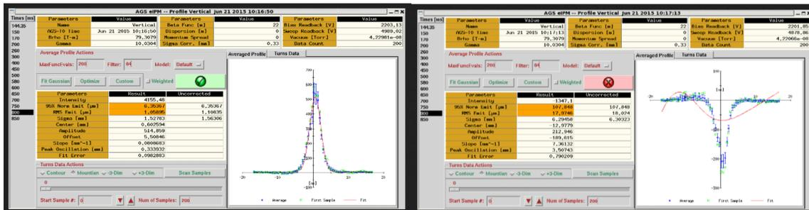
The "negative profiles" were not a problem during proton fills when only one bunch was injected in each AGS cycle. However when several bunches were injected the individual bunch profiles interfered with each other and dramatically reduced the average profile. During the shutdown we removed the output transformers to dc couple the amplifiers to the digitizers. This eliminated the "negative" profiles and provided good profile measurements with heavy-ion operation.
