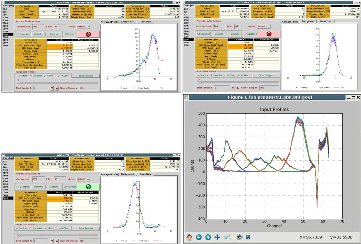
We constructed approximate gain correction values for channels 10-48 from the scan. Below is a calibration scan after these first corrections were applied. Also are profiles after corrections at the same times as those above. The profile at 3.0s is Gaussian and the beam sigmas decrease as the beam is accelerated.
