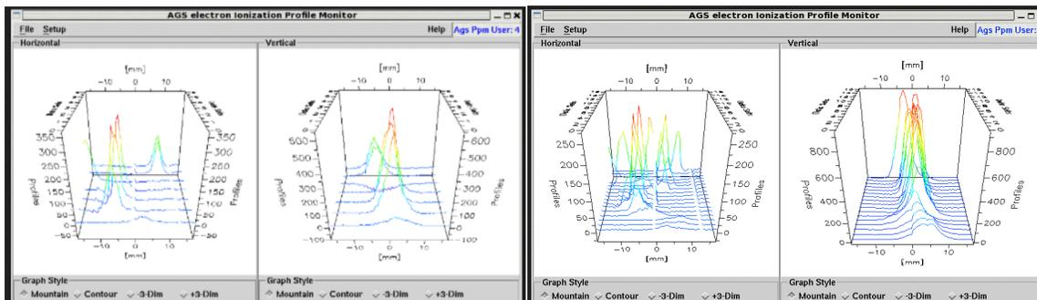
Once we were aware of the measurement artifacts arising when the beam was near the dead zone boundary we were able to understand that this was the cause of strange behavior of the horizontal eIPM. Dedicated measurements showed that the AGS orbit in the horizontal IPM was consistently below beam line center, in the direction of the MCP. During the Run 15-16 shutdown we flipped over the horizontal eIPM detector to place the 'dead zone' at the top of the chamber.
