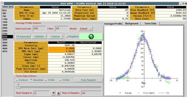
Profiles of Au beam at injection energy, April 15
