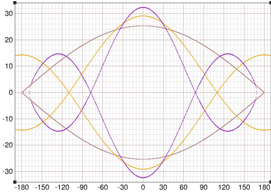
Figure 12: As in the previous figure, the brown and orange curves are the single and double-harmonic buckets for the case in which the amplitude ratio A_1/A_2 is fixed at 15/22 . As the harmonic 3h amplitude, A_3 , is raised from zero, the double-harmonic bucket becomes a triple-harmonic bucket. The area of this bucket will decrease from \mathcal{A}_3 = \mathcal{A}_2 to a minimum and then begin to increase. The value of R which gives the minimum area can be read off from Figure 8 . There one finds R = 1.994 . The corresponding unstable fixed point phase \phi_u obtained from Figure 9 is 77.633 degrees. The corresponding bucket area ratio \mathcal{A}_3/\mathcal{A}_1 obtained from Figure 10 is 0.532 . The violet curve is the minimum-area triple-harmonic bucket.
