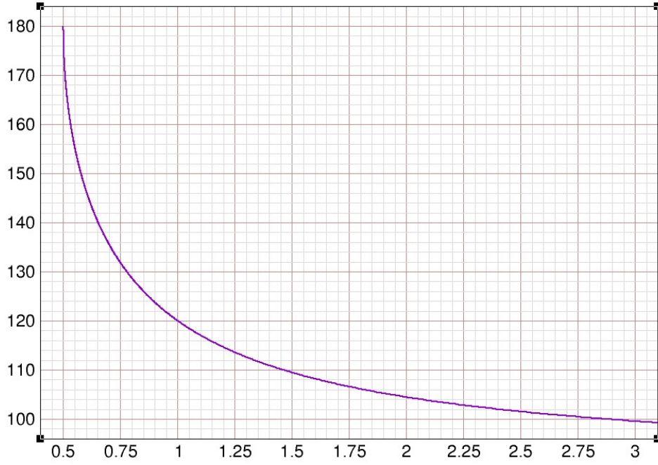
Figure 6: Double-harmonic bucket unstable fixed point phase \phi_u versus voltage ratio V_2/V_1 . This follows from equation (72).
