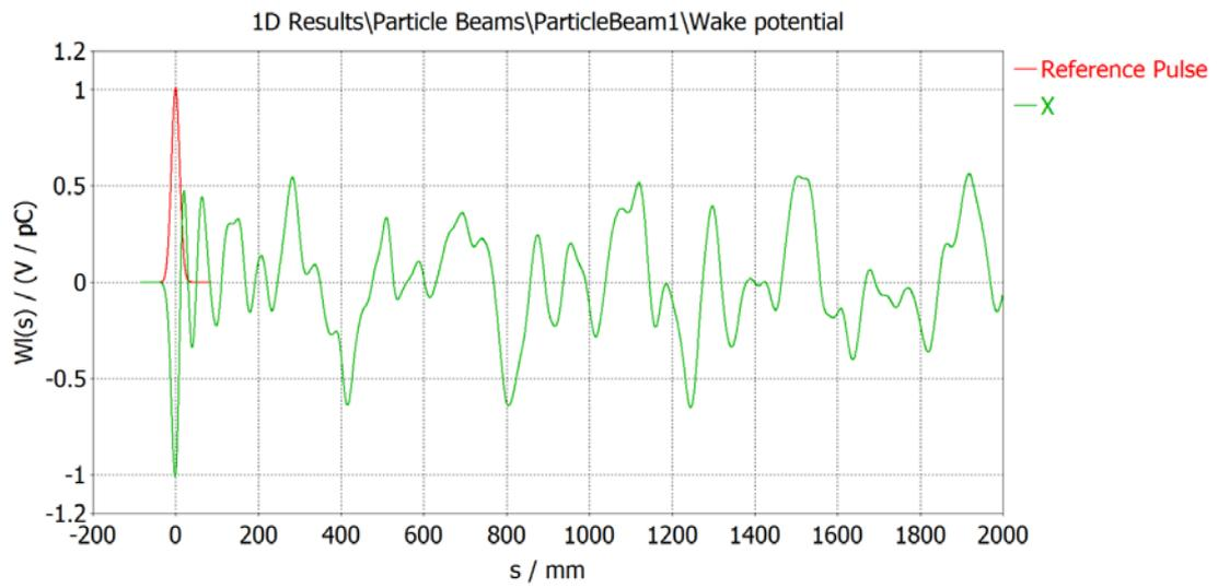
Figure 7: The longitudinal wake potential for the booster cavity with  $\beta=1$ .
