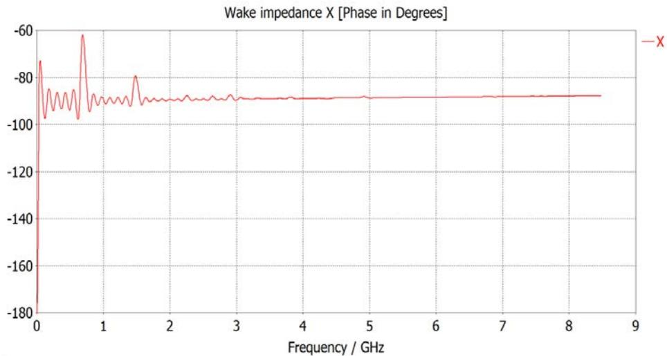
Figure 11: The phase of the longitudinal impedance.
