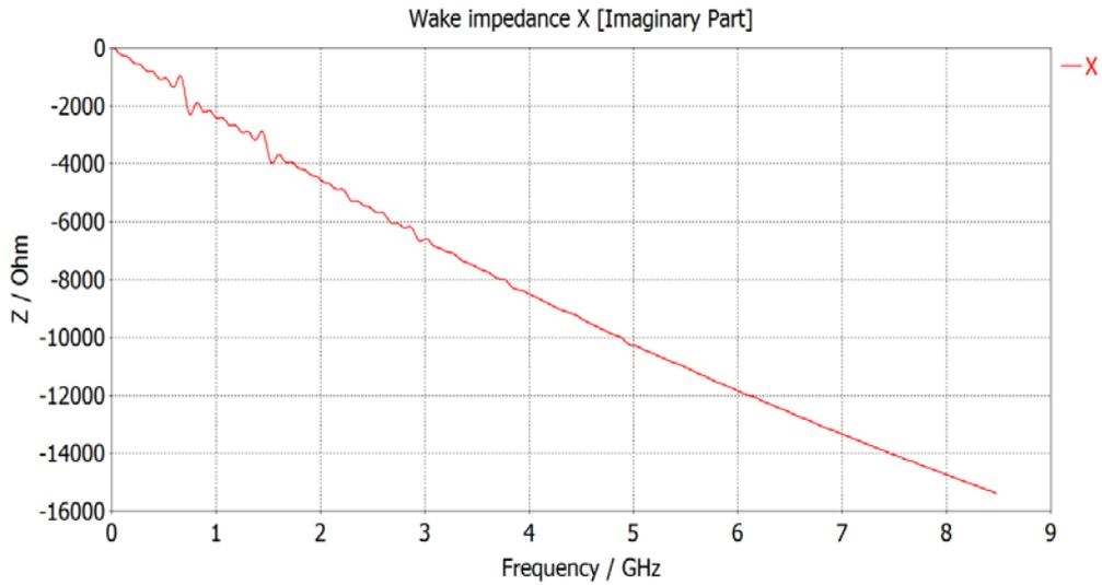
Figure 10: The imaginary part of the longitudinal impedance.
