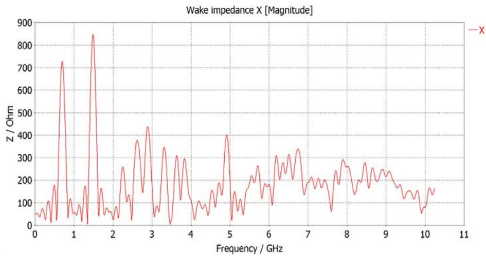
Figure 8: The longitudinal impedance of the booster cavity.
