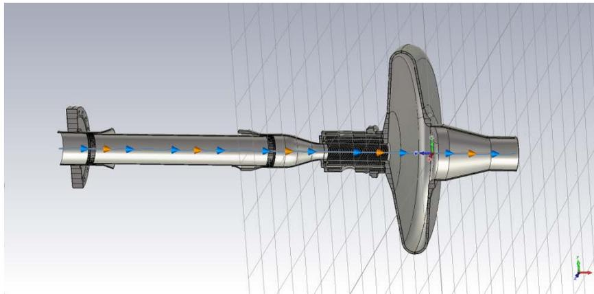
Figure 3: Simplified booster cavity structure in CST simulation.
