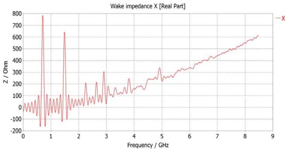
Figure 9: The real part of the longitudinal impedance.
