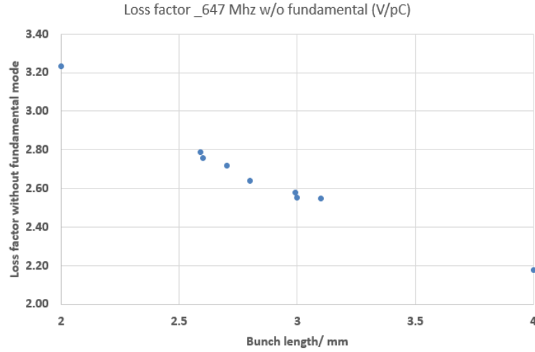
Figure 2: Integrated loss factors of the 647 MHz 5-cell BNL4 cavity for different rms bunch length.
