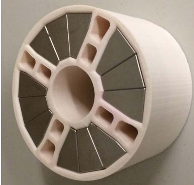
Figure 8. A picture of the actual modified Halbach quadrupole. The housing of the permanent magnet wedges is made by a 3D printer.
