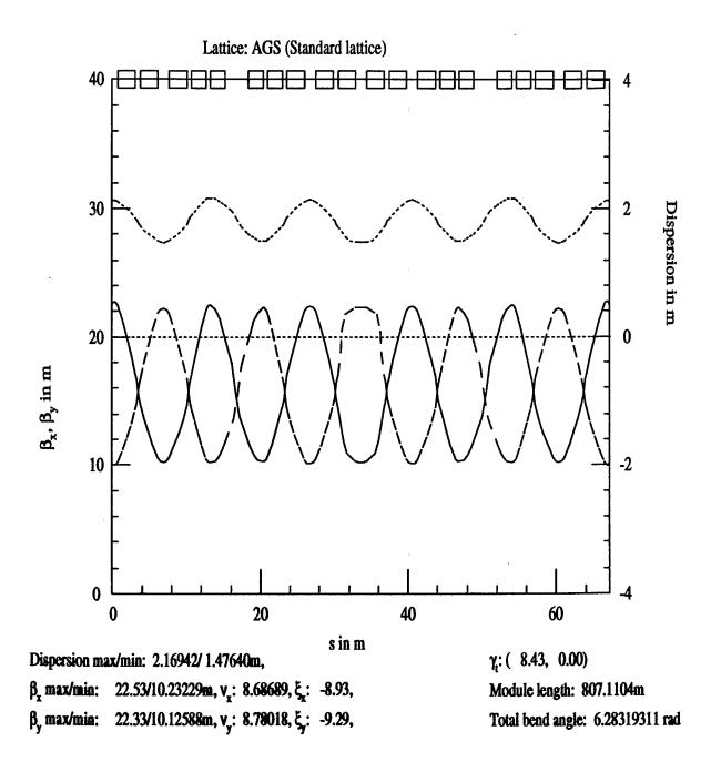
Figure 1: Orbit Functions in standard AGS Lattice
