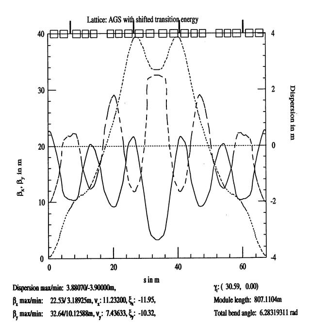
Figure 2: Orbit Functions in AGS lattice with shifted magnets and quads
