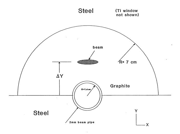
Fig. 1 Schematic View of the Dump Face
