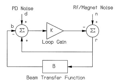
Fig.1 Block diagram of a beam phase feedback loop.
