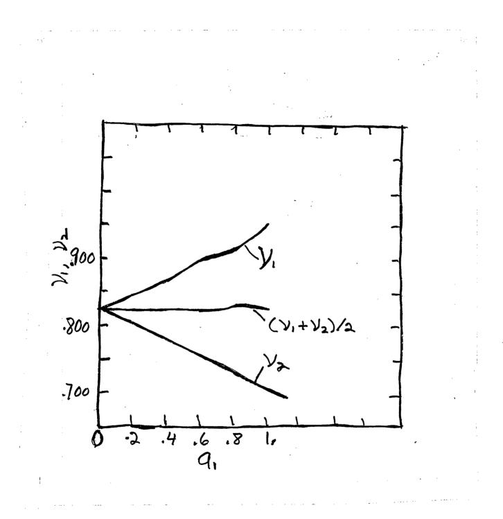
**Figure 1:** A plot of the normal mode tunes,  $\nu_1$  and  $\nu_2$ , versus the size of the random skew quadrupole error,  $a_1$  for a particular distribution of the random  $a_1$ . The tune splitting was not corrected.
