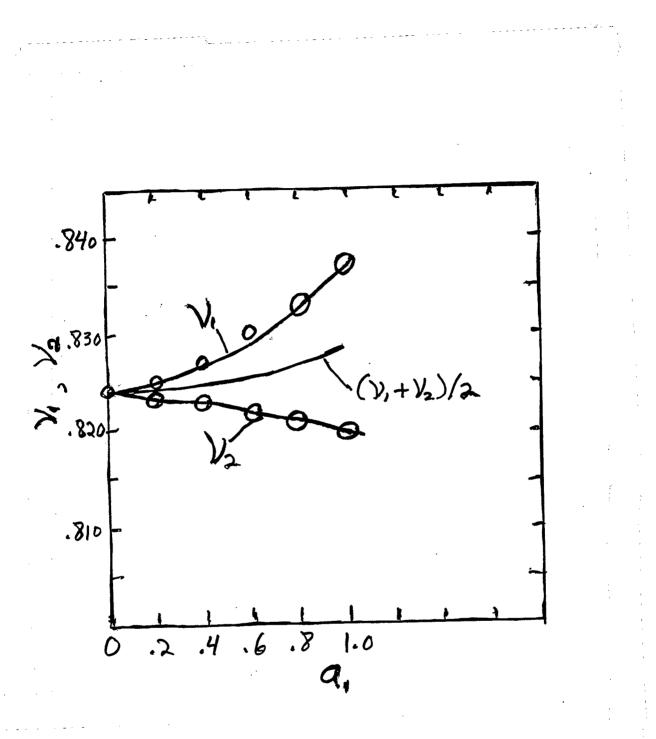
**Figure 2:** A plot of the normal mode tunes,  $\nu_1$  and  $\nu_2$  versus the size of the random skew quadrupole error,  $a_1$ . The tune splitting has been corrected with the 2 family correction system. The open circles show the points on an  $a_1^{3/2}$  curve.
