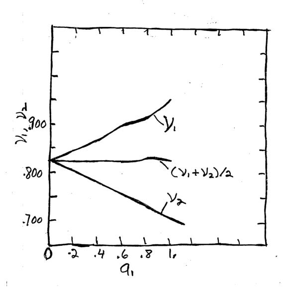
Figure 1: A plot of the normal mode tunes,  $\nu_1$  and  $\nu_2$ , versus the size of the random skew quadrupole error,  $a_1$  for a particular distribution of the random  $a_1$ . The tune splitting was not corrected.
