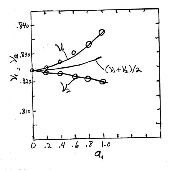
Figure 2: A plot of the normal mode tunes,  $\nu_1$  and  $\nu_2$  versus the size of the random skew quadrupole error,  $a_1$ . The tune splitting has been corrected with the 2 family correction system. The open circles show the points on an  $a_1^{3/2}$  curve.
