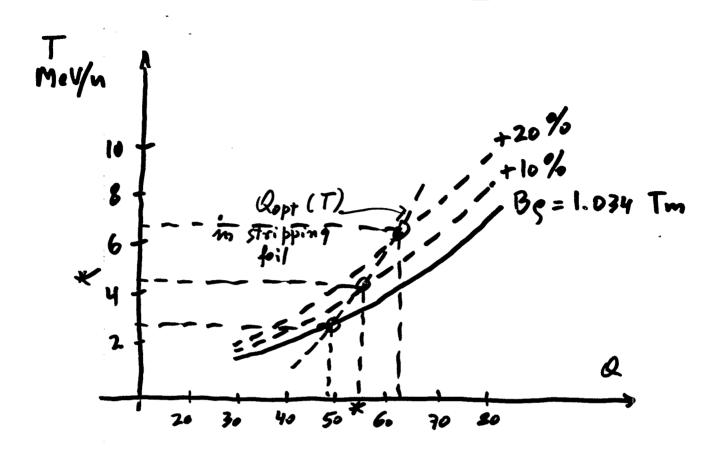
DESIRED : • AS HIGH A CHARGE STATE AS POSSIBLE TO INCREASE SPS INJECTION ENERGY AND REJUCE # OF HARMONIC JUMPS
