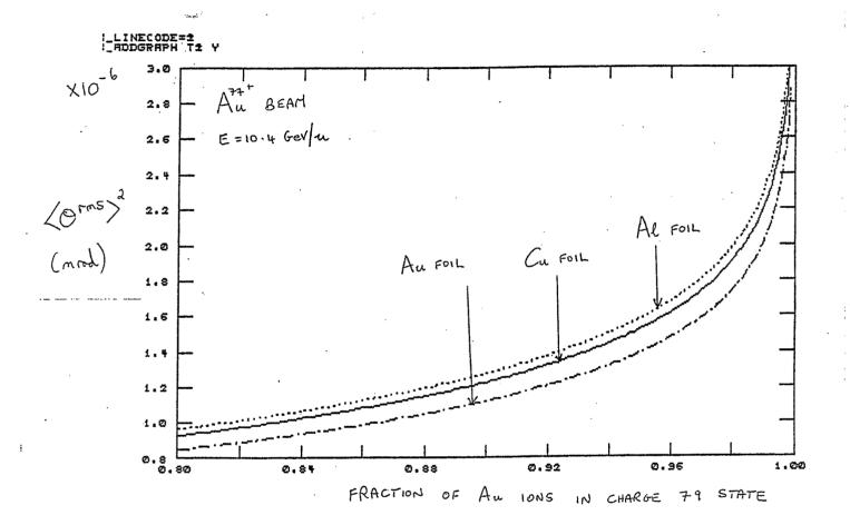
Fig. 3 Plot of the angular spread  $(\theta^{rms})^2$  as a fraction of fully stripped Au ions for Al, Cu and Au foils.
