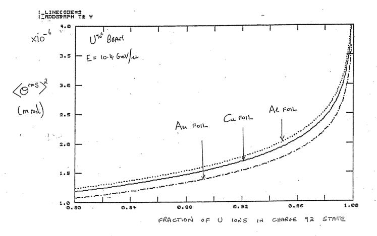
Fig. 4 Plot of the angular spread  $(\theta^{rms})^2$  as a fraction of fully stripped U ions for Al, Cu and Au foils.
