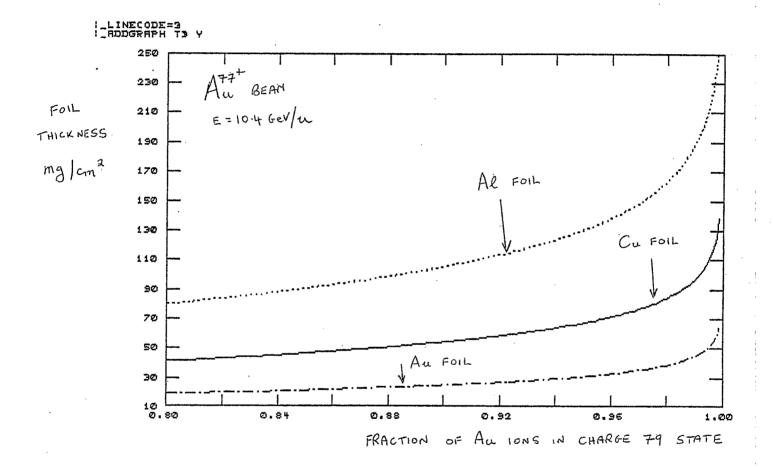
Fig. 1 Plot of the required foil thickness as a fraction of fully stripped Au ions for Al, Cu and Au foils.
