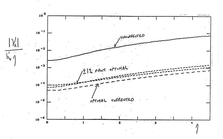
Fig. 3 Plot of the x,y component of  $\nu^{(4)}/b'_4\eta$  as a function of  $\eta$ . The corrected values are shown for the modified corrector scheme when  $b'_{QF} = b'_{QD}$ .
