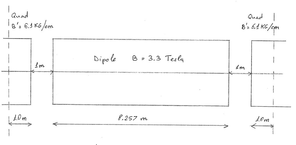
No. of Dipoles / Ring = 192 No. of Quads / Ring = 192 Special Dipoles and Quads not included
