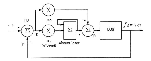
Fig.2A digital PLL block diagram with improved stability.
