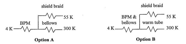
Abbreviations are given under <u>parameters</u>. A simple heat balance is taken at the junction to solve for the temperature there. Heat loads out of the junction to 4K (end volume) and 55K (heat shield pipe) follow. The thermal conductivity integrals are as given in Technical Note # 327 in the BNL Cryogenic Data Reference. The geometrical parameters are given. The equation to be solved is as follows (for option A):
