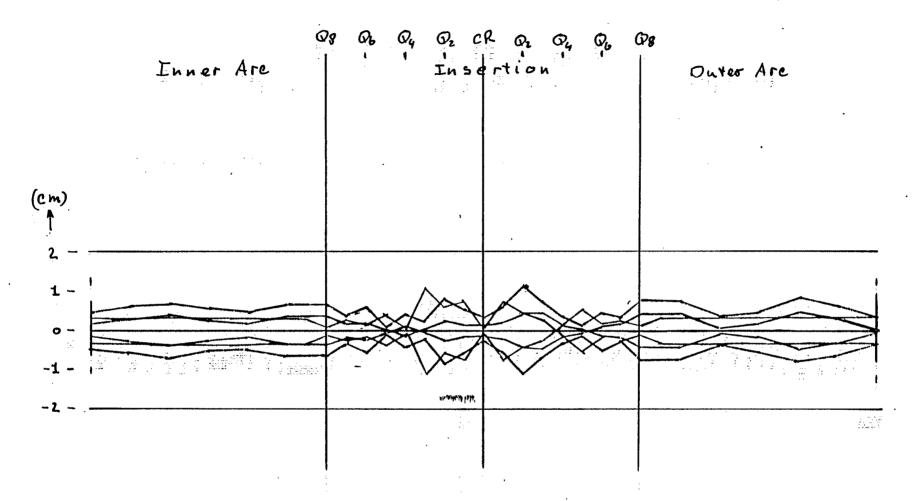
Beam dimensions after 2 hrs at f = 100 $\varepsilon = 18.4 \times 10^{6} \text{ Nad-m } (2.50)$  $\frac{410}{10} = \pm 2 \times 10^{-3}$
