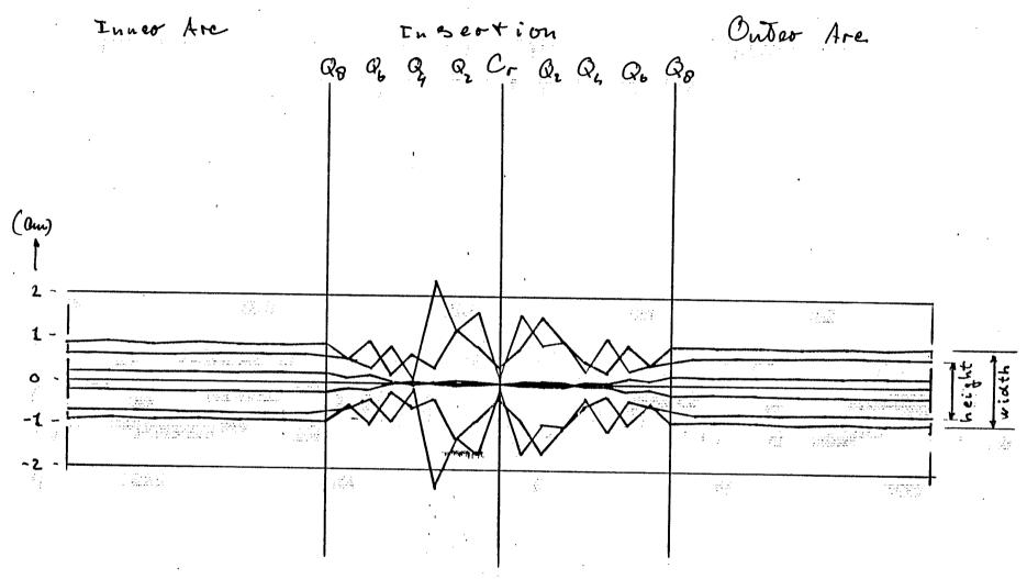
Beam dimensions at injection f = 12  $\Sigma = 10 \times 10^{6} \text{ rad-m} (2.50)$   $\frac{\Delta P}{P} = \pm 1.62 \times 10^{-3}$
