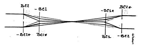
± BC1, ± BC2, ± BC1\*, ± BC2\* are dipoles with parallel entrance and exit edges, ± indicates polarity.
