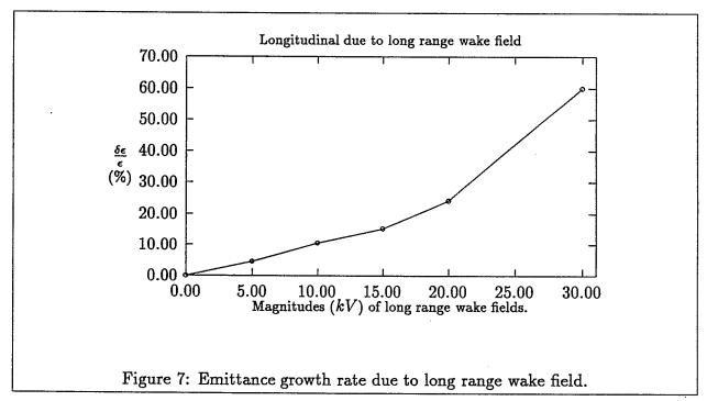
The larger the emittance of a bunch in the accelerating bucket, the harder it is to transfer the bunch into the storage bucket. The transfer scheme is to adiabatically lower the voltage
