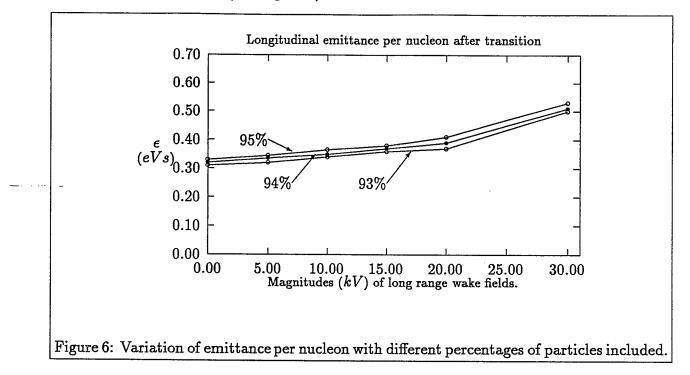
Naturally, to find the emittance growth rate due to long range wake field, we need only to compare the emittance at different magnitudes of induced voltage to that when induced voltage is zero. Note 95% of the particles are used in the definition of the emittance.
