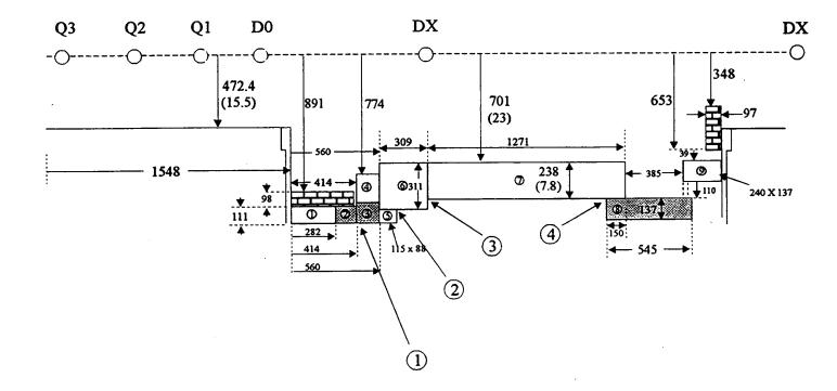
This drawing is the CASIM approximation of the BRAHMS shield wall at elevations below 10 ft. Engineering drawings dated April 25 1997.
