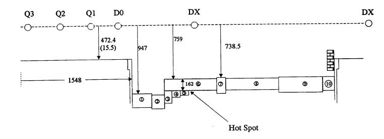
This drawing is the CASIM approximation of the BRAHMS shield wall at elevation 78 ft. 8 in.. Engineering drawing Sept. 1997.
