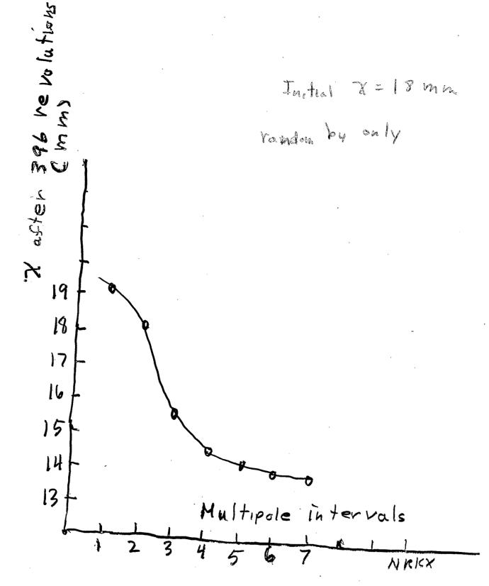
Distributed Maltipole Results Increasing the humber of intervals to describe the multipoles changes results -significantly However, As (the Stability limit) is not changed. Occasionally Assis increased by 2mm for some runs. Point multipoles appear to give essentially the correct result for Asi
