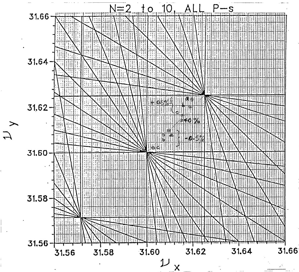
Table IV.- Variation of momentum with amplitud with resolution of 100 turns. Points a, b, c represent emittances  $0, 1.5\pi \times 10^{-6} \text{ m-rad}$ ,  $3\pi \times 10^{-6} \text{ m-rad}$  respectively. We kept chromaticity 1 in order to avoid 8th and 10th order resonances.
