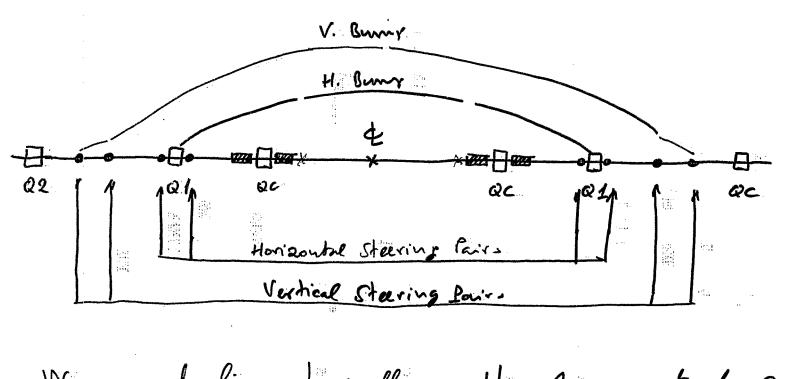
We are dealing Lerically with 2-magnet local bumps, though for convenience in practice the system is made of 4-magnets -
