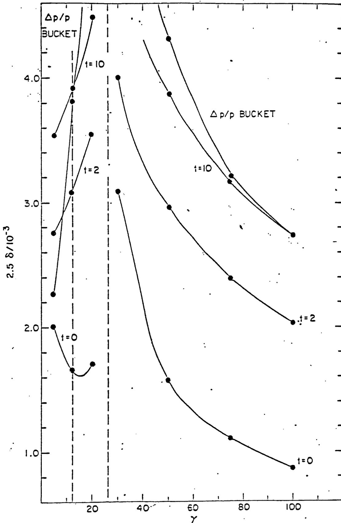
Beam bunch height growth due to intra-beam scattering.
