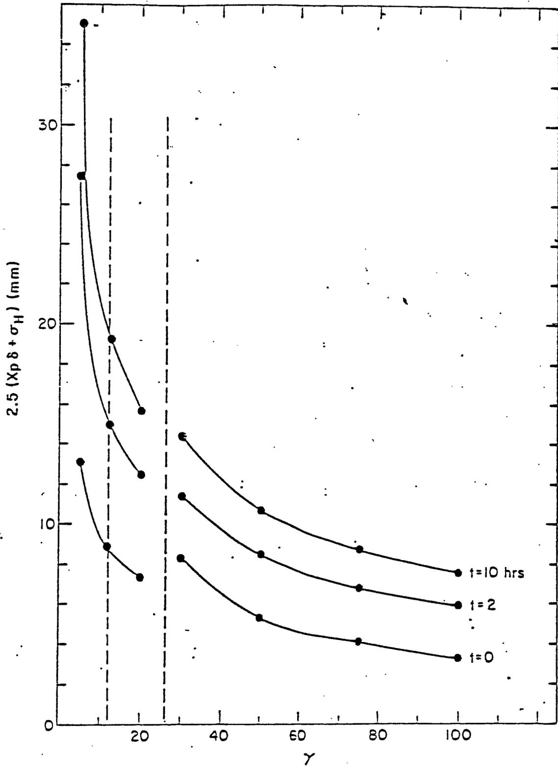
Beam half-width growth due to intra-beam scattering.
