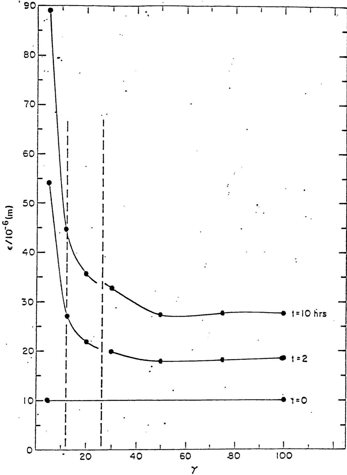
Beam emittance growth due to intra-beam scattering.
