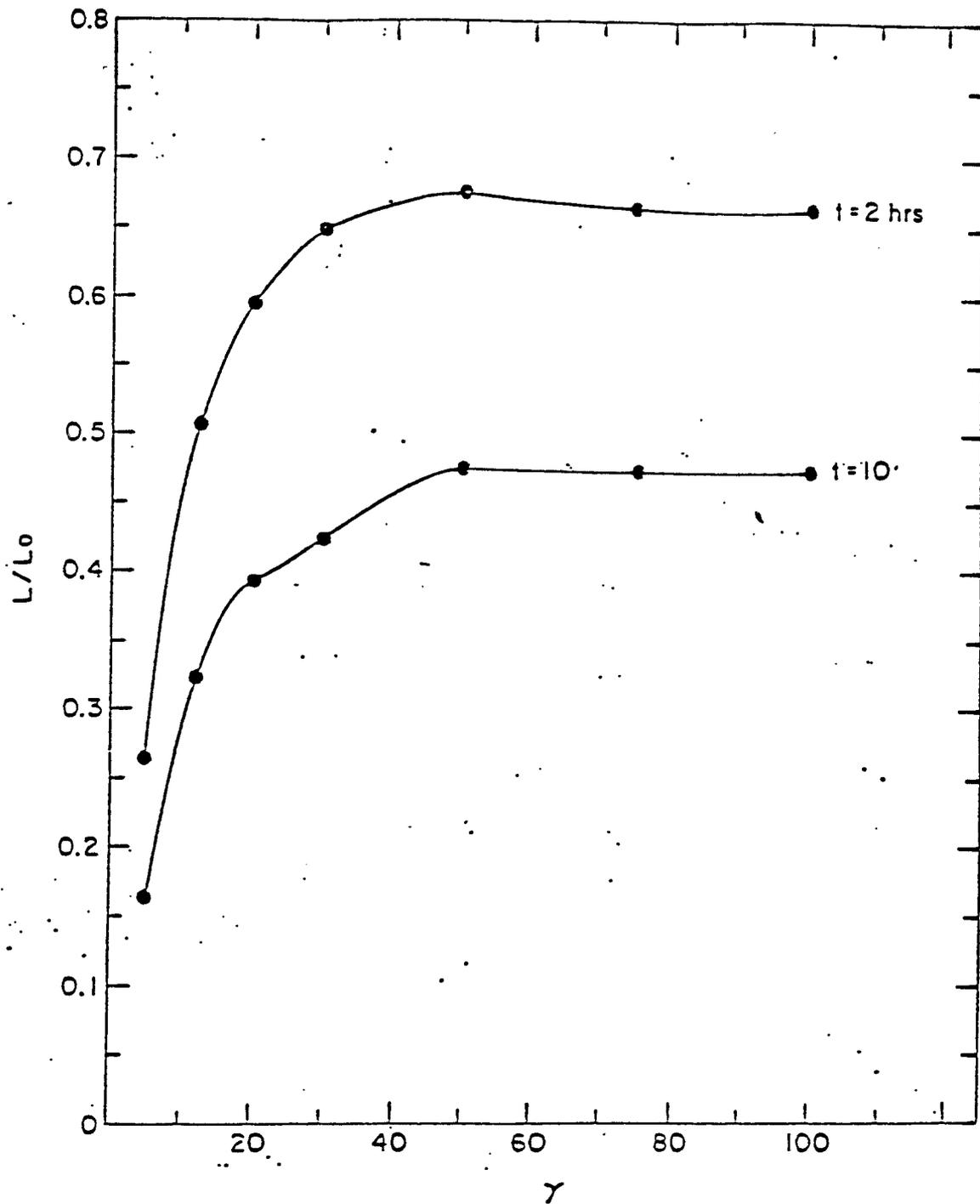
Average luminosity (normalized to its initial value) versus energy for the case of Au on Au, and head-on collisions.
