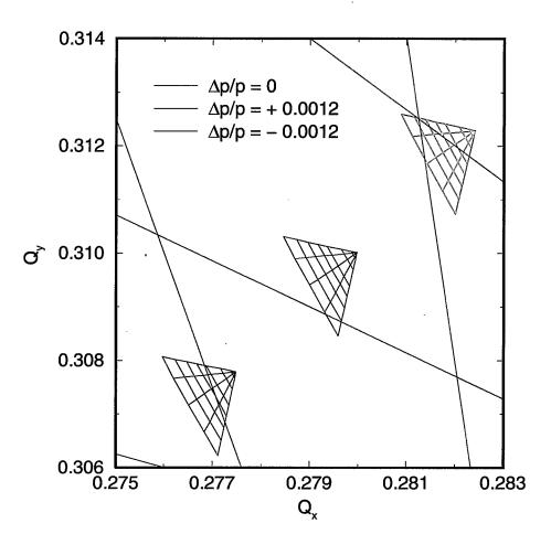
Ideal LHC operating point at injection (Tune spread for up to  $11\sigma_{x,y}$  particles;  $\Phi = 0$ )
