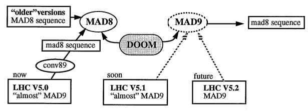
DOOM among its other services provides a bridge between MAD8 and MAD9. It is important to notice that MAD9 will support a way to generate MAD8 sequences, if desired, so that the conversion program conv89 can be phased out when MAD9 will be fully developed and operational. Existing LHC related software in the US comprises:
