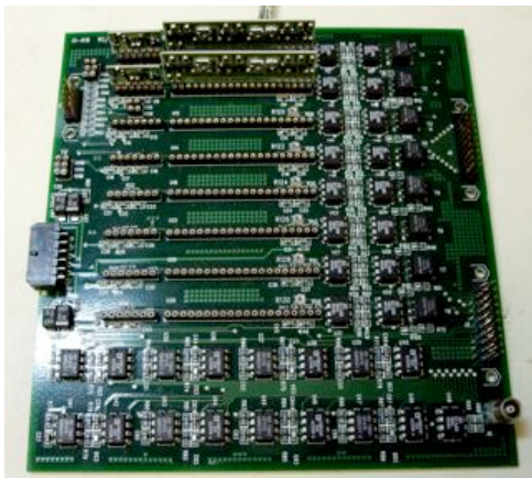
Figure 4. An 8-channel amplifier board. Two of the fast channels, top, are shown populated with the hybrid charge and shaper amps.
