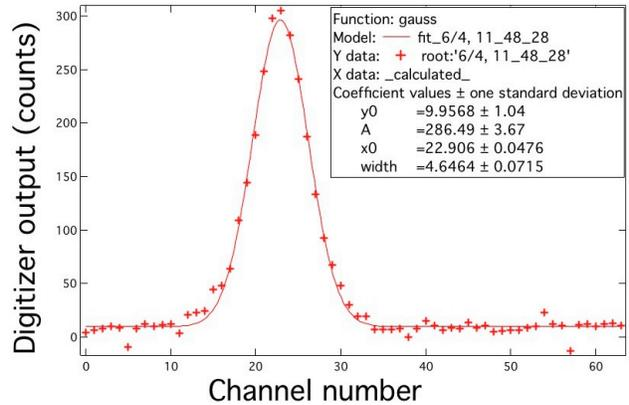
Figure 5. Beam profile during the acceleration ramp
