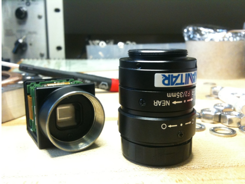
Figure 2.35 - Flea 2 camera along with ThorLabs MVL35M23 lens. Note that the cover of the camera body has been removed in order to aid in evacuation of the camera chamber and prevention of trapped volumes.
