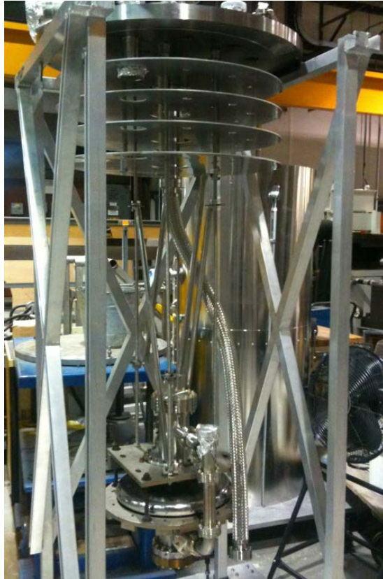
Figure 2.24 - Photograph of the cavity attached to the top plate during initial test preparations. The top plate rests on a support frame, and the cavity is suspended from the top plate by support rods that pass through the four baffle plates. In addition, a flexible vacuum hose, not shown in the picture, attaches to the cavity and passes through the baffles.
