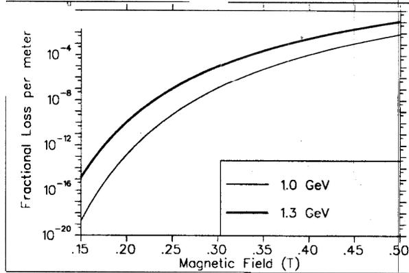
Figure 1: Fractional H<sup>-</sup> stripping loss per meter as a function of magnetic field.
