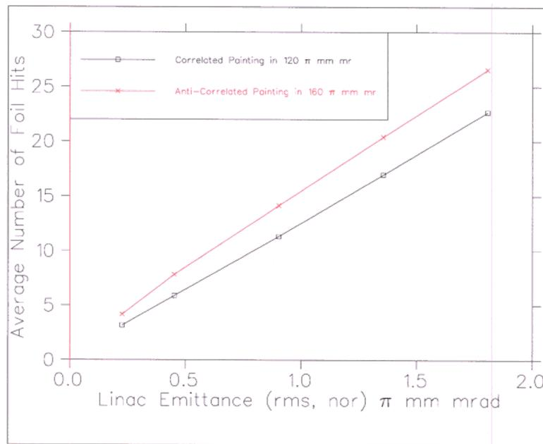
Figure 5: Average number of foil hits during the accumulation (1225 turns) as a function of linac emittance. For the correlated option the painted phase space area is  $120 \pi$  mm mrad and for anti-correlated painting, the phase space area is  $160 \pi$  mm mrad.
