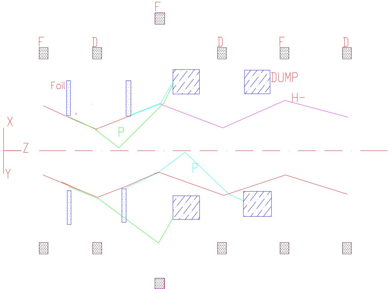
Figure 2: Schematic of the HEBT Collimator configuration.
