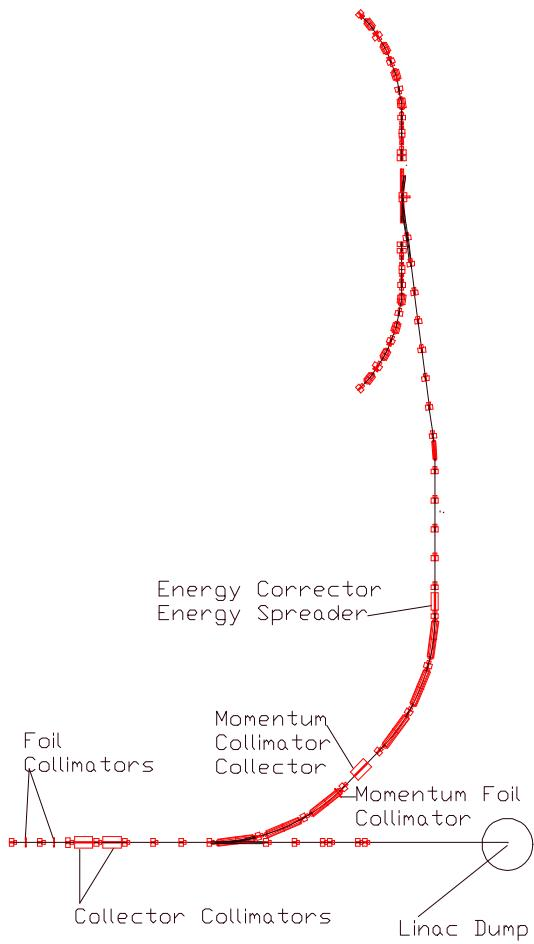
Figure 1: Layout of the HEBT line.
