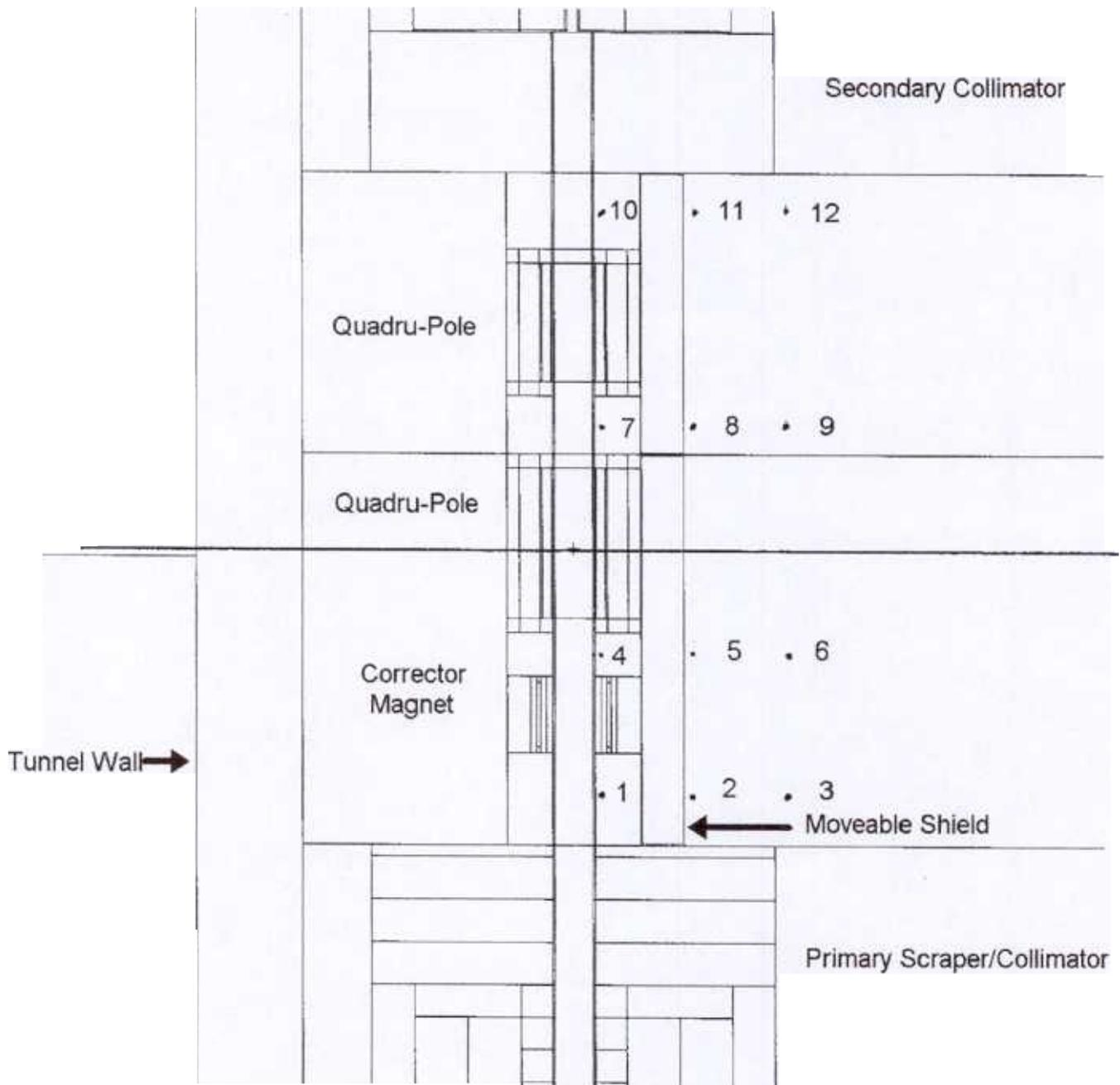
Figure 7: Location of Detectors - Moveable Shield Parallel to Beam Direction (Full Length)
