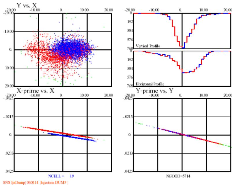
Figure 10B: Particle distribution at Injection Dump for three times the design emittance and mismatched. **Red** particles representing particle started at foil as  $H^-$ , **Blue**  $H^0$  and **Green** as lost particles in the flight tube.
