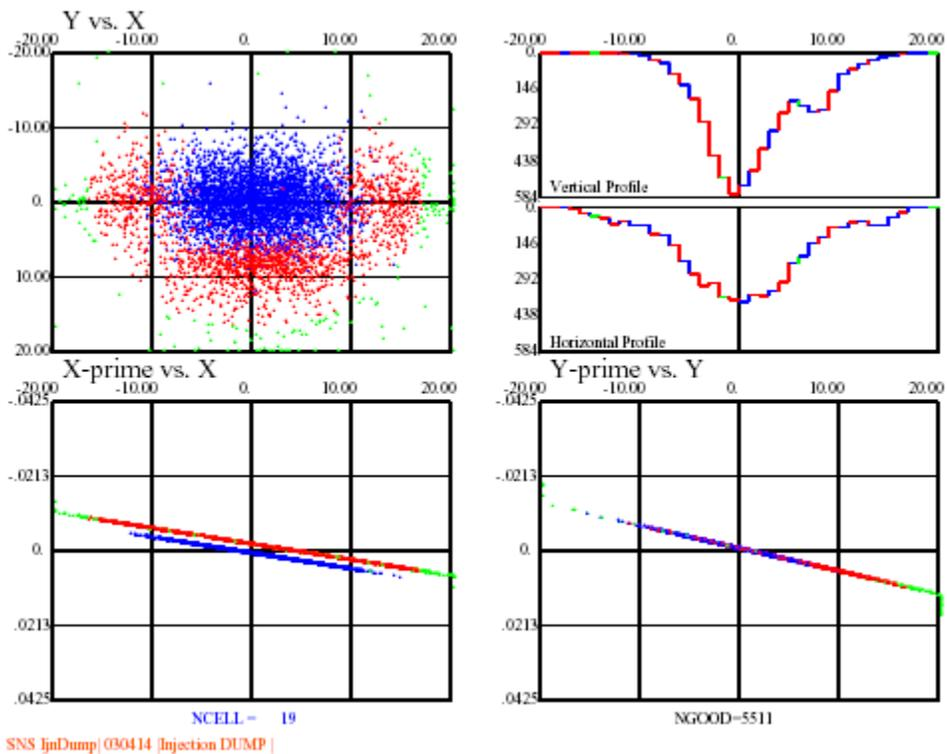
Figure 7B: Particle distribution at Injection Dump for two times the design emittance and matched. **Red** particles representing particle started at foil as  $H^-$ , **Blue**  $H^0$  and **Green** as lost particles in the flight tube.
