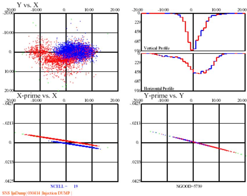
Figure 9B: Particle distribution at Injection Dump for two times the design emittance and mismatched. **Red** particles representing particle started at foil as  $H^-$ , **Blue**  $H^0$  and **Green** as lost particles in the flight tube.
