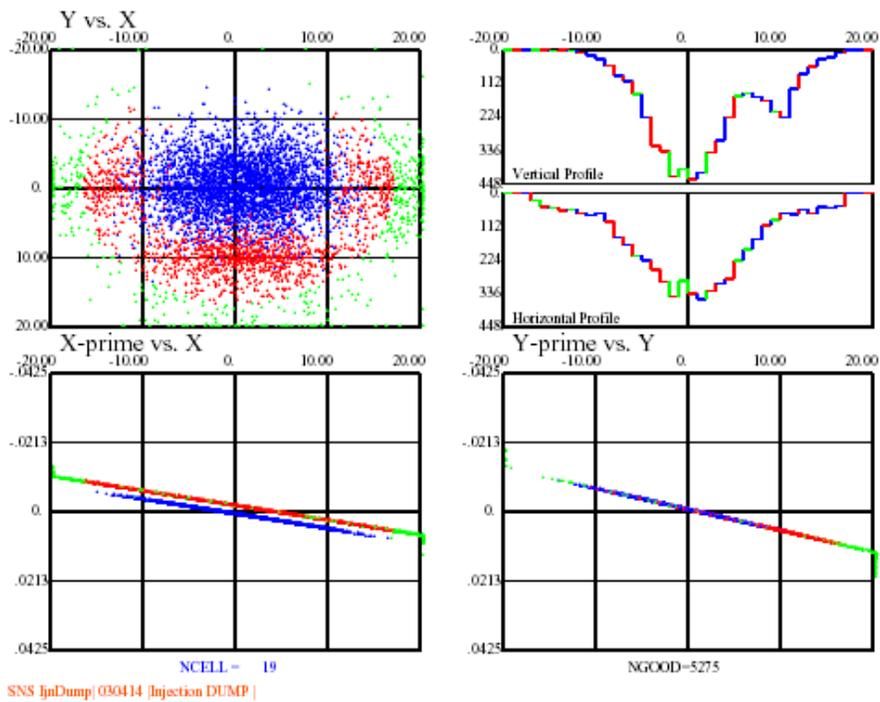
Figure 8B: Particle distribution at Injection Dump for three times the design emittance and matched. **Red** particles representing particle started at foil as  $H^-$ , **Blue**  $H^0$  and **Green** as lost particles in the flight tube.
