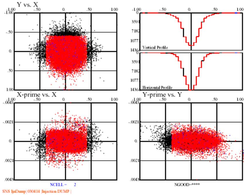
Figure 10A: Particle distribution at the foil for three times the design emittance and mismatched injection. **Red** particles representing P, **Black**  $H^-$  and **Blue**  $H^0$ .
