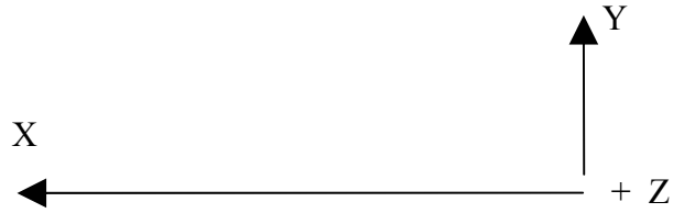
Figure 1: The coordinate system used. X is radial, away from the center of the ring. Z is into the paper in the clockwise direction around the accumulator ring.
