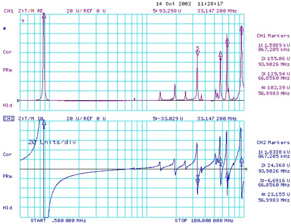
Fig.1. Coupling impedance of SNS cavity with open ceramic rings
