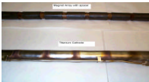
Fig.1. Magnetron and Titanium target
