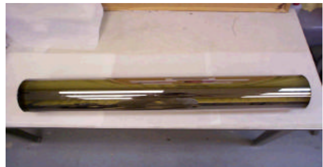
Fig. 5b. #2 glass tube with grounding Al stripes
