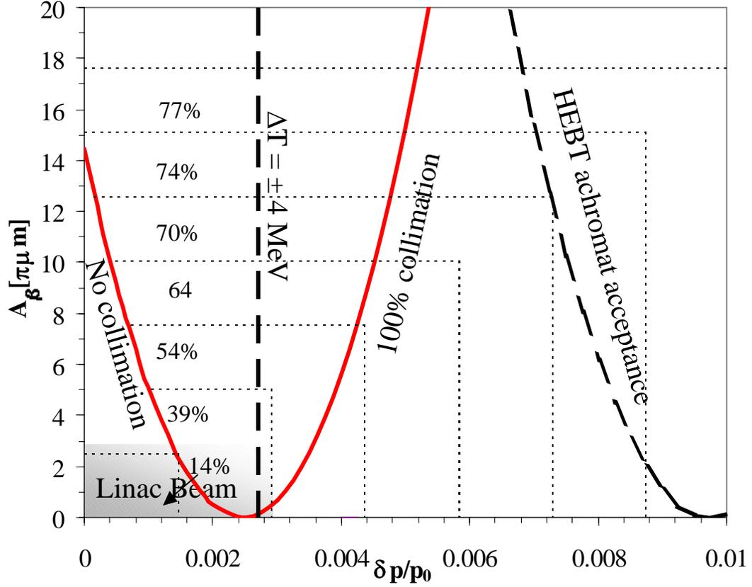
Figure 7: Collimator acceptance in terms of betatron amplitude vs.  $\delta p/p_0$ . The geometry acceptance of the HEBT achromat and the momentum spread limit at  $\pm 4$  MeV are represented by dashed lines.
