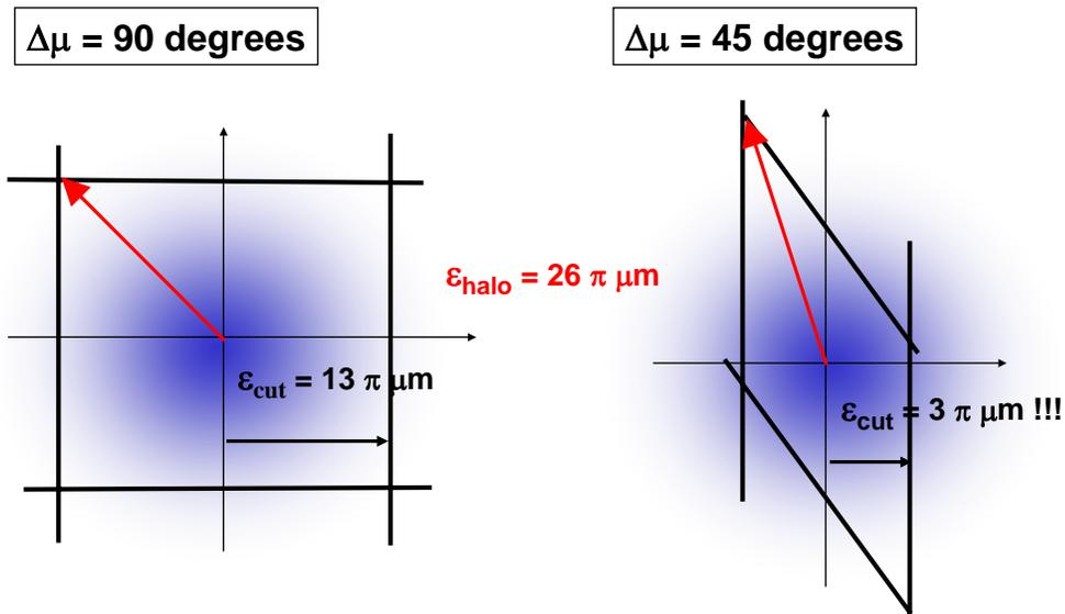
Figure 2: Cuts induced by the striper foils in normalized phase-space for two systems at 90 and 45 degrees of phase advance, respectively. The maximum extent of the escaping halo is required to be  $26\pi\text{mm}\cdot\text{mrad}$  in both cases.
