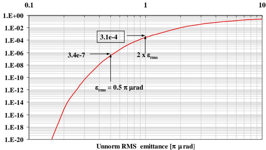
Figure 1: Fraction of the beam exceeding a fixed aperture in the HEBT line. The aperture is chosen to match  $13\pi\text{mm}\cdot\text{mrad}$ , half of the HEBT acceptance and equal to the collimator acceptance.
