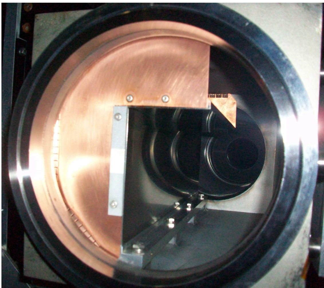
Figure 4: Recently inspected Yellow primary collimator, showing a flat surface without any damage.
