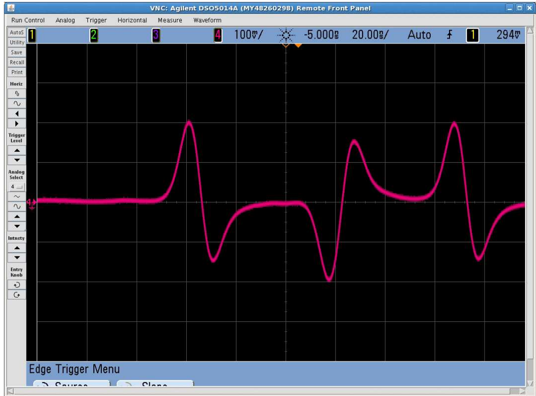
Figure 2: Scope image depicting the raw signal from an IP8 DX BPM, Jun 22 2011.
