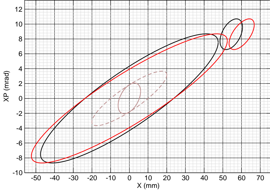
Figure 12: Here, as before, the large and small black ellipses are the machine and beam ellipses, respectively, at the inflector exit. These evolve into the red ellipses in the 0.64253 meter drift from the inflector exit to quadrupole QHC4 of the Booster lattice. The half-aperture of the quadrupole is 76 mm. The incoming beam ellipse has parameters A = 0 and B = 0.3 and emittance \pi\epsilon_0 = 11\pi mm milliradians. It ends up safely inside the QHC4 quadrupole aperture. The black machine ellipse is centered on the Booster beam pipe and just touches the septum of the inflector. The outer side of the 1 mm thick septum is 48.5 mm from the center of the beam pipe. The solid brown ellipse is the incoming beam ellipse shifted to the center of the machine ellipse. The dashed brown ellipse is the smallest machine ellipse that contains the beam ellipse. It is well inside the black machine ellipse.
