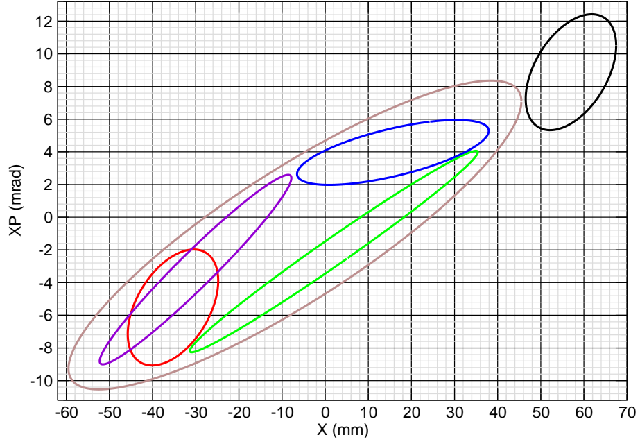
Figure 28: The black, red, green, blue, and violet curves are the beam ellipse after 0, 5, 6, 7, and 8 turns, respectively, from launch time 2.0 turns. The large brown ellipse is the machine ellipse that just touches the inflector septum. Its area is 248.290 \pi mm milliradians which may be taken to be the acceptance of the machine. The initial (black) ellipse launched at time 2.0 turns therefore ends up inside the machine acceptance after the bump has collapsed.
